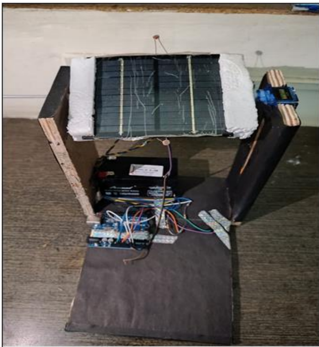
Fig 1 Working Model of Solar Tracking System
