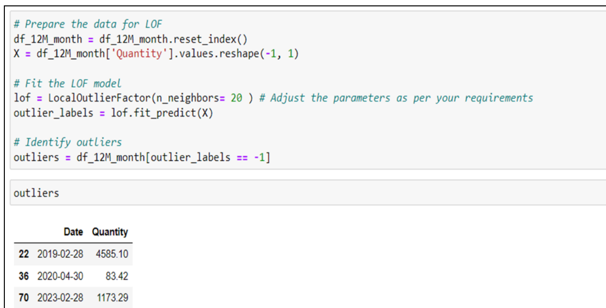
Fig. 9: LOF-Based Outlier Detection: Illustrating Identified Anomalies
