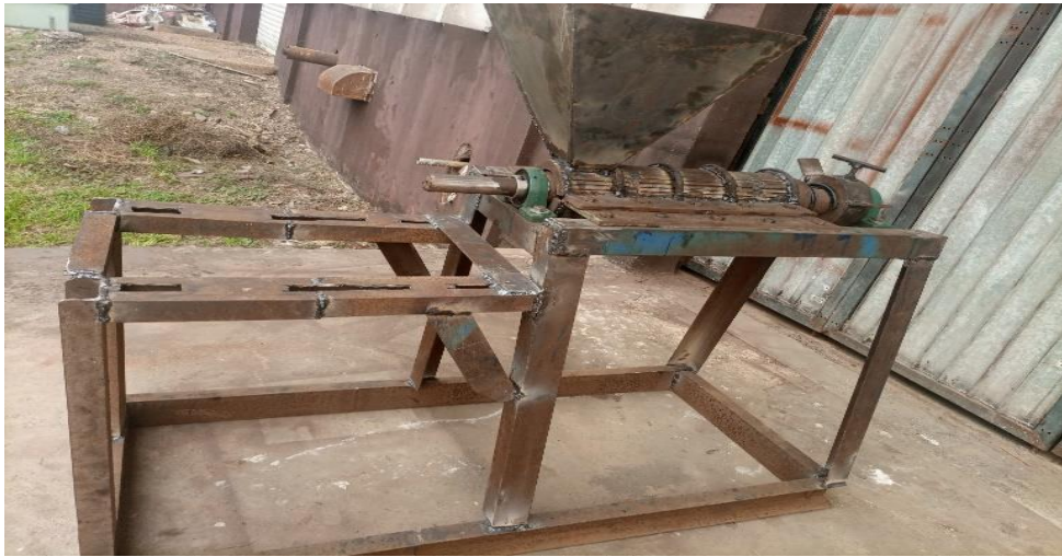
Fig. 17: Pictorial view showing the foundation coupling along with components of the upper chamber
