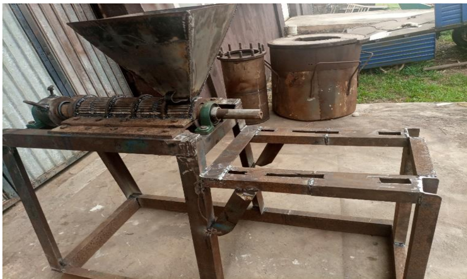
Fig. 16: Pictorial view of barrel, foundation bolts and gear motor sit
