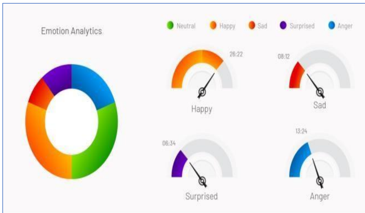
Fig. 8: The above pie chart shows the overall breakdown of the emotions displayed by the user. This report is further enhanced by the speed-o-meter of the various emotions. This will show the total time per emotion during a session, and then percent value of the same
