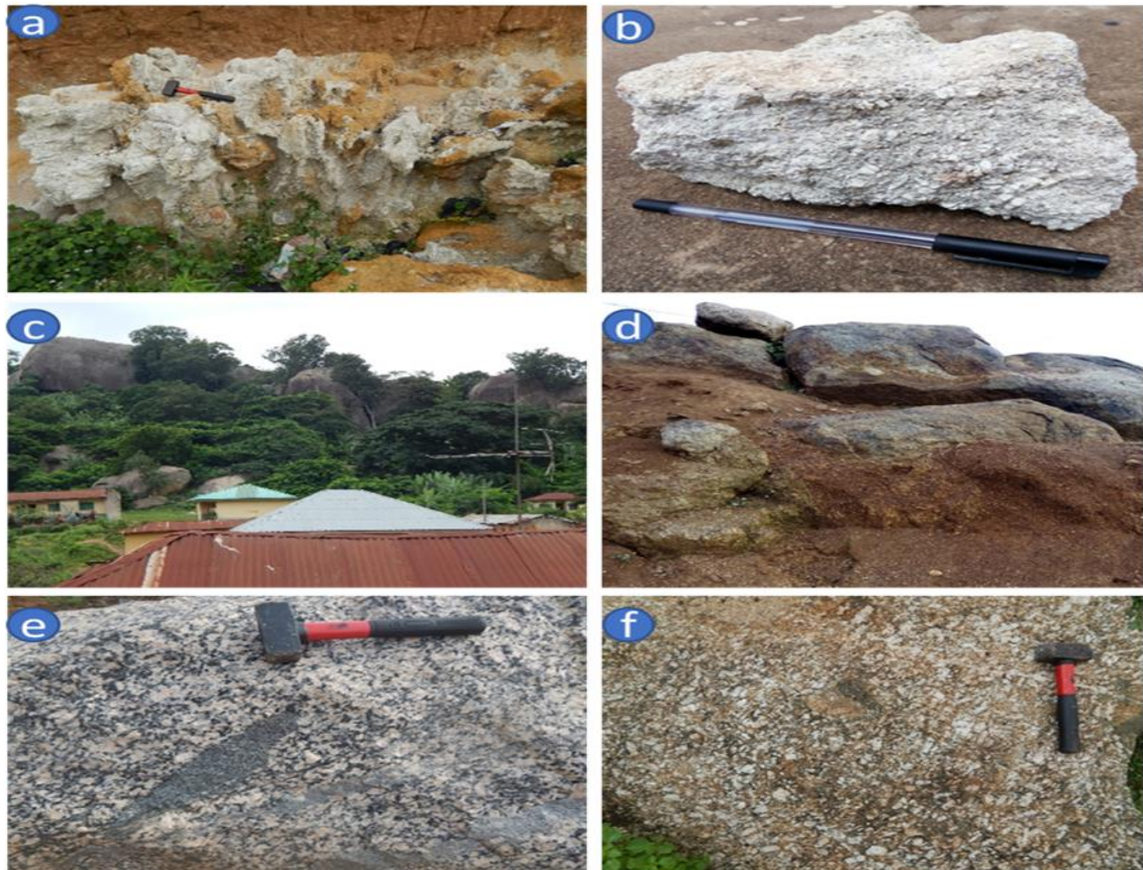
Fig 7 Impact of Chemical Weathering on Rocks in the Study Area (a) Extensive Exposure of Saproelite (b) Hand Specimen Sample of the Saproelite with Faintly Recognizable Feldspar Porphyries, (c) Extensive Outcrop of Charonockite Chattered into Boulders by Physical Weathering, (d) Chemically Altered In-Situ Charonockite Exposed in Dallimore Area, Ado-Ekiti (e) Fresh and Unaltered Granite Outcrop, (f) Early Stage of Chemical Weathering in Granite from the Study Area (the Characteristic Pink Feldspars have Changed to White and the Rock became Soft with a Hollow Sound when Struck with a Hammer).
