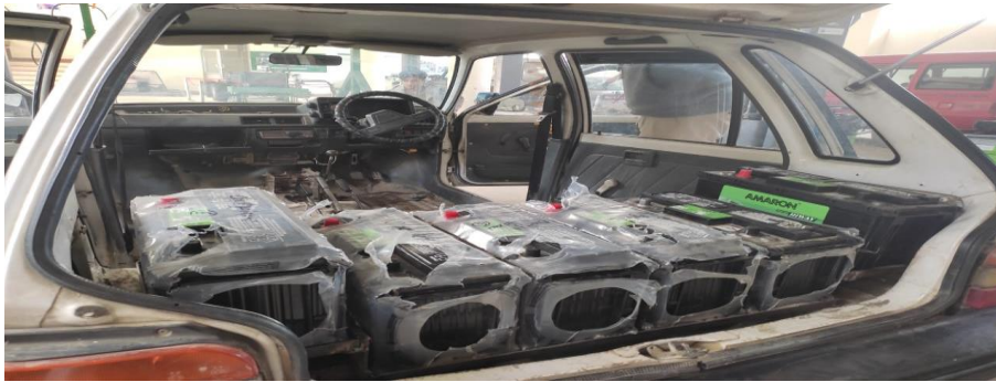
Fig. 17: Battery system installed under the hood
