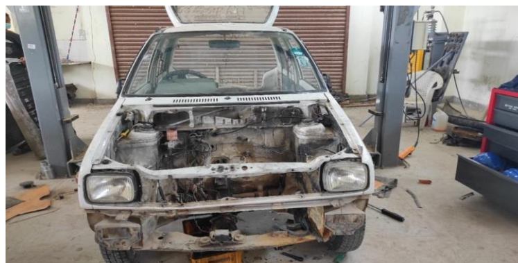
Fig. 2: Frontal part of the disassembled car
