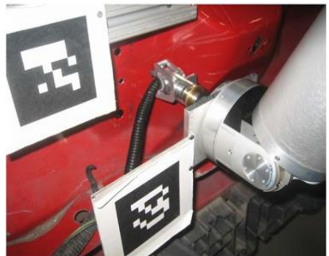
Fig 2 The Plug is Moved Toward the Target by the Arm.
