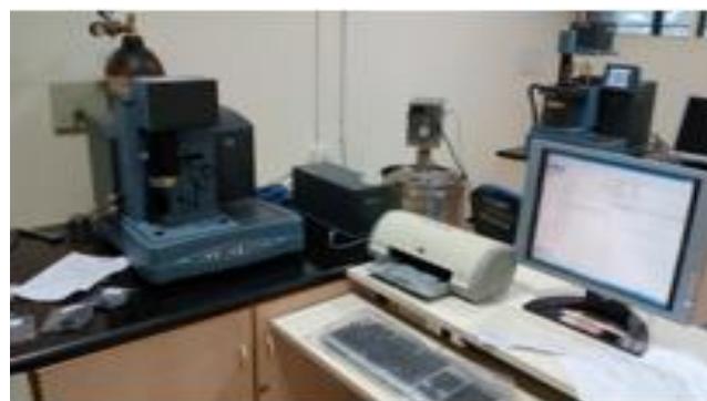
Fig 2 Experimental Set Up used for Thermogravimetric Analysis (Universal V 4.7 TA Instrument)
