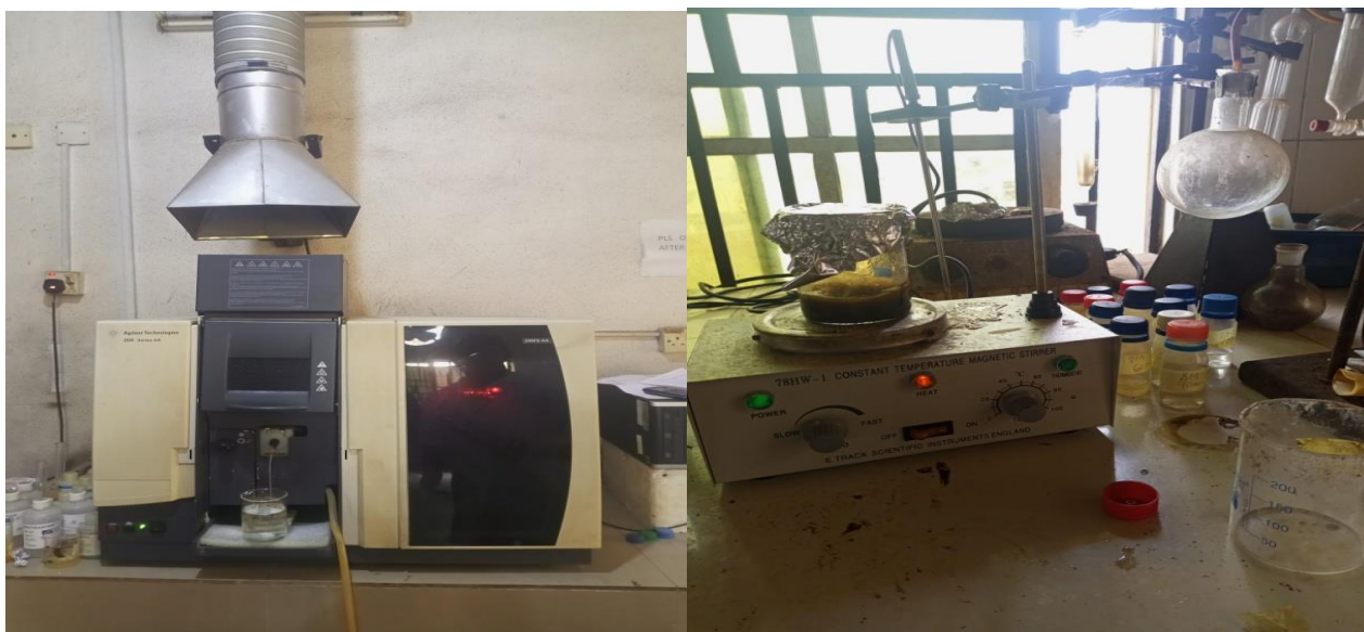
Fig 3 (a)Atomic Adsorption (b)Sample on a Hot magnetic Spectrophotometer (AAS) Stirrer
