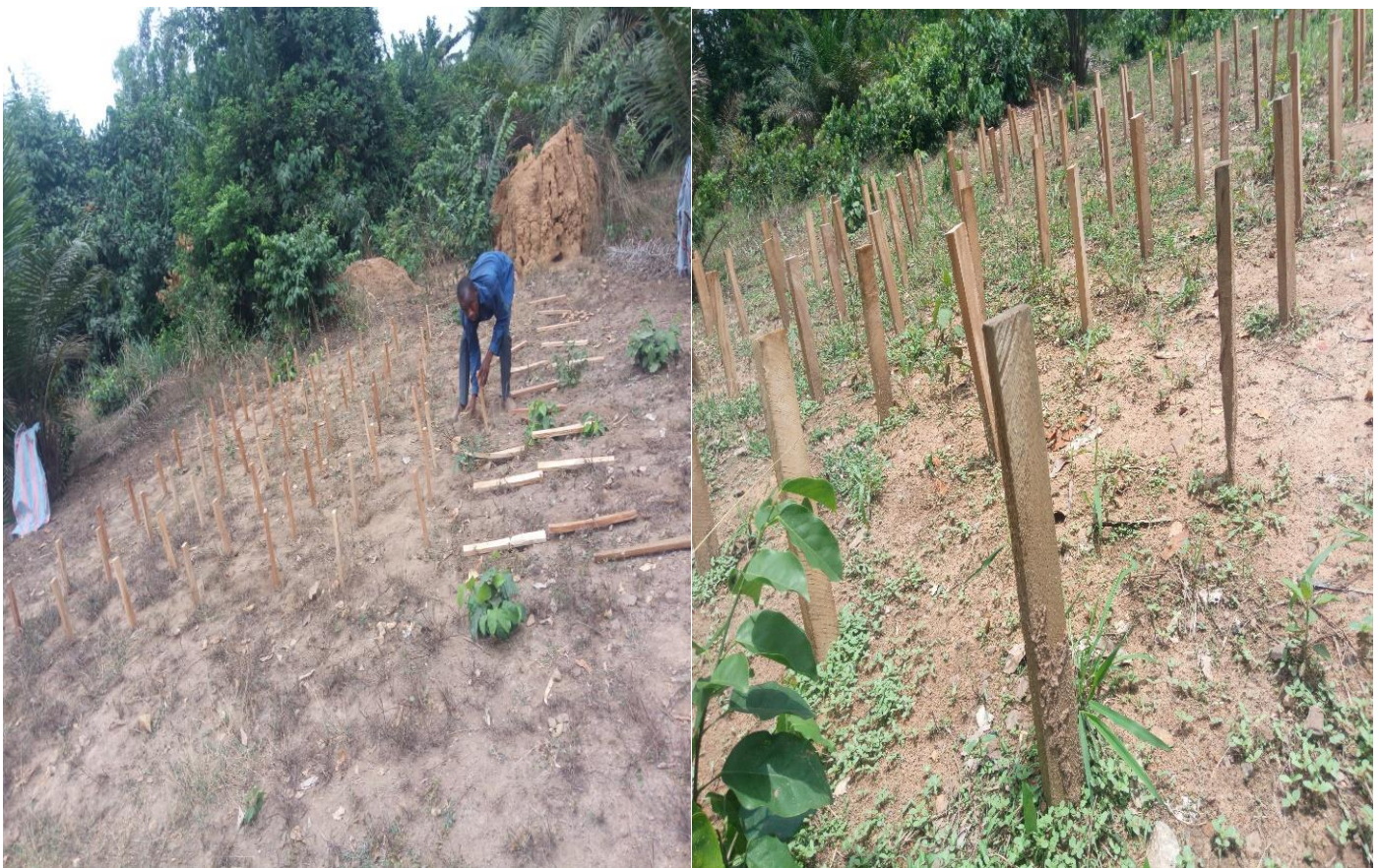
Fig 1. above shows the specimen being mounted at the Demonstration field to determine the level of natural resistance of neem to termites and other biodegradation factors at the Kwame Nkrumah University of Science and Technology test site.
