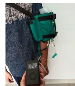
Fig 4. Inflating the balloon of Digital Mobile Infusion Bag using a digital pum
