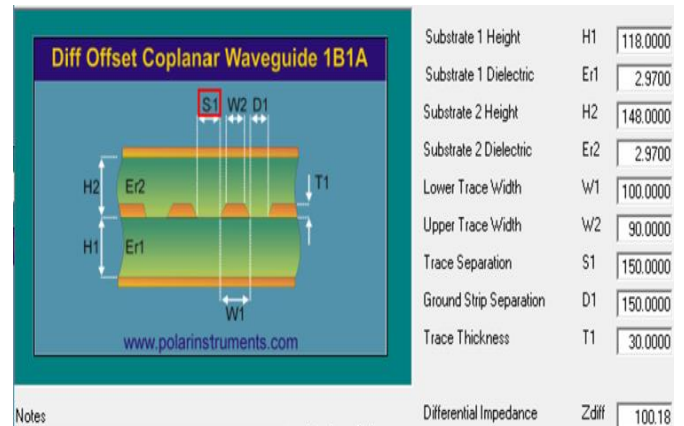
Fig 24 100-ohm Impedance with Stripline
