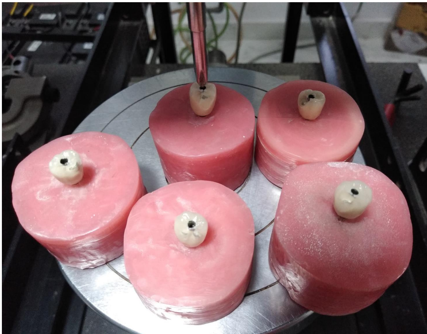
Fig 7 Fractured Specimen Under Instron Machine
