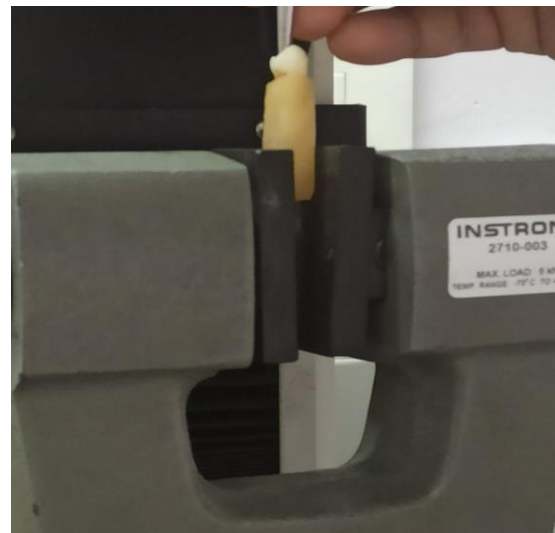
Fig 1 Stationary Compressive Load Applied using Universal Testing Machine on the Occlusal Surface.
