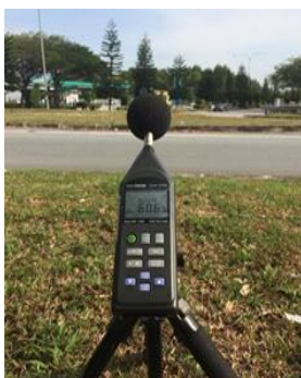
Fig 3 Installation of Sound Level Metre (SLM)
