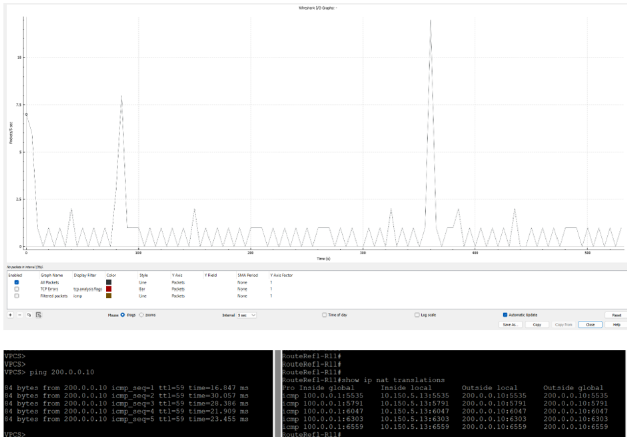
Fig. 5: Ping results from clients to internet with I/O graph in Wireshark
