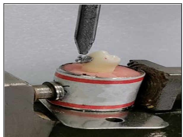
Fig 3: Measuring Shear Bond Strength using Instron Machine
