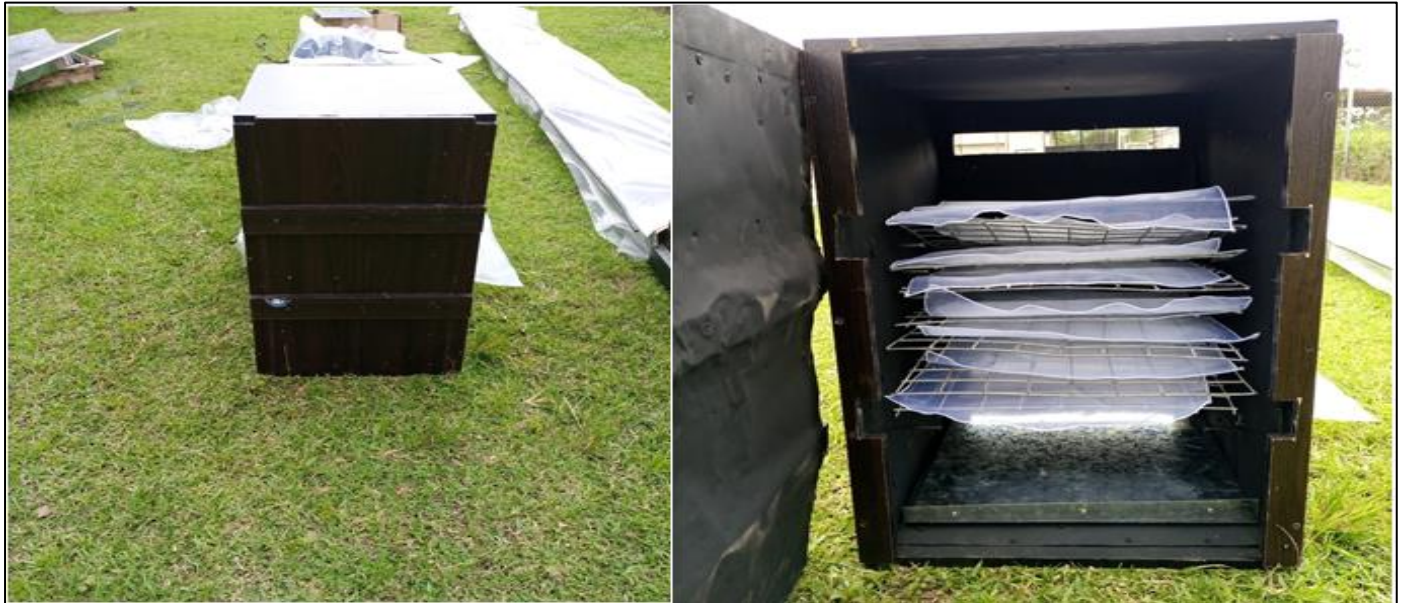
Plate 2 Showing the Layers of the Seven Trays in Drying Chamber
