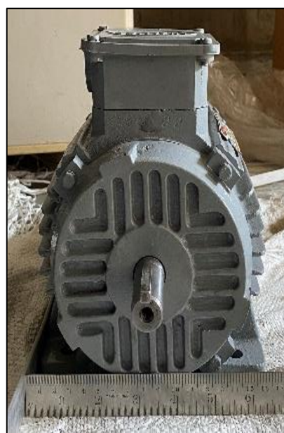
Fig 2 3-phase Induction Motor
