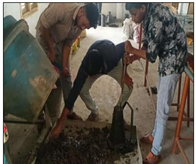
Fig 7: Concrete Mixing and Slump Cone test
