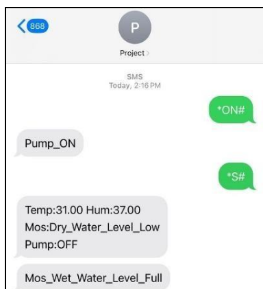
Fig 18 Alert Sent to Indicate that Water Level is Full / Soil is Wet
