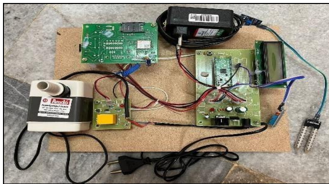
Fig 11 Designing Cost-Effective SMS based Irrigation System using GSM Module
