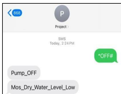
Fig 17 Alert Sent to Indicate that Water Level is Low / Soil is Dry
