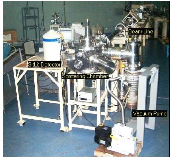
Fig 1: The Ion-Beam Facility Setup at Institute of Physics (IOP), Bhubaneswar, India for the PIXE measurements.
