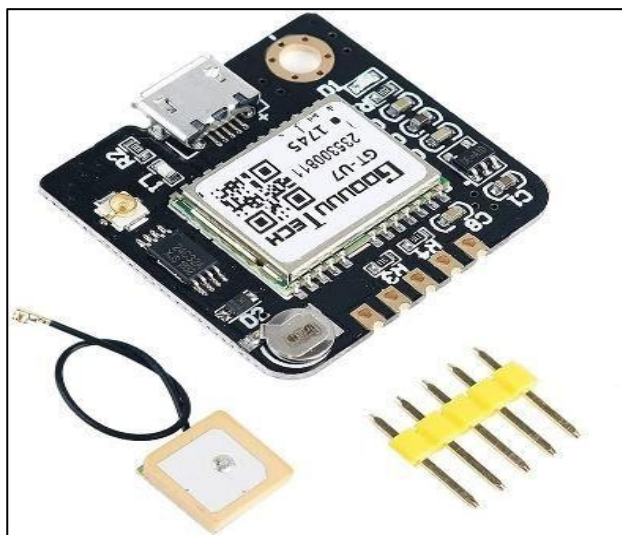
Fig 7: GPS Module for Location Tracking
