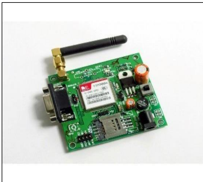
Fig 6: GSM Module for Alerting Authorities
