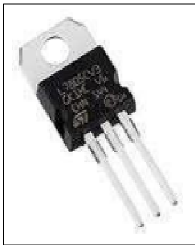
Fig 7 7805 IC Voltage Regulator
