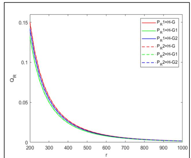
Fig 9: Simulation Curves of Received Power Per Unit Area with Distance under Different Combinations of Scattering Phase Functions
