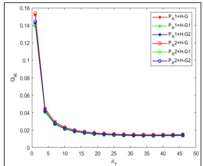
Fig 12: The Simulation Curve of the Received Power Per Unit Area with the Change of the Transmitting Half Field Angle Under the Combination of Scattering Phase Function
