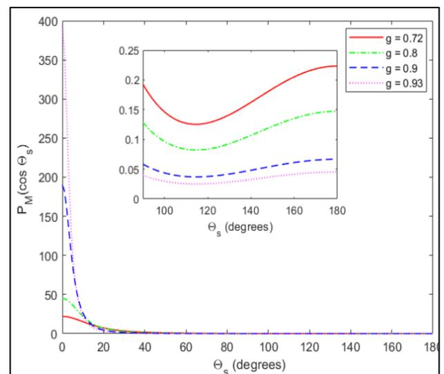
Fig 6: Mie Scattering Phase Function ( H-G2 ) under Different Weather Conditions
