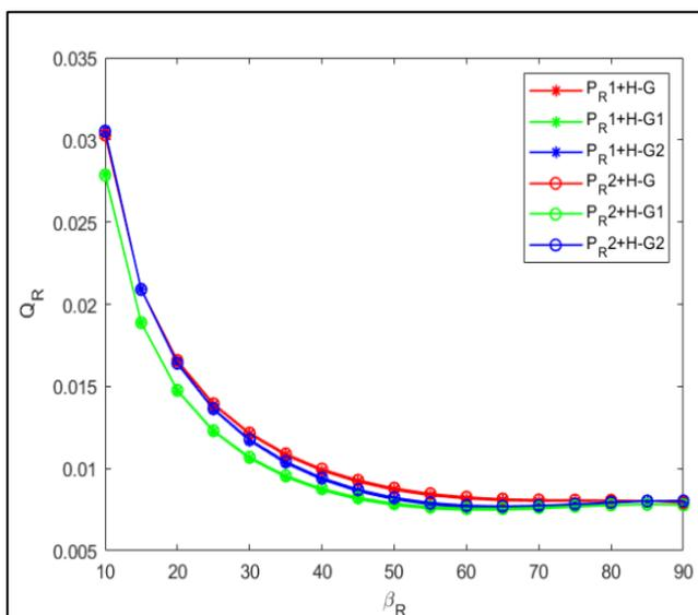
Fig 11: The Simulation Curve of the Received Power Per Unit Area with the Change of the Receiving Elevation Angle under Different Scattering Phase Function Combinations
