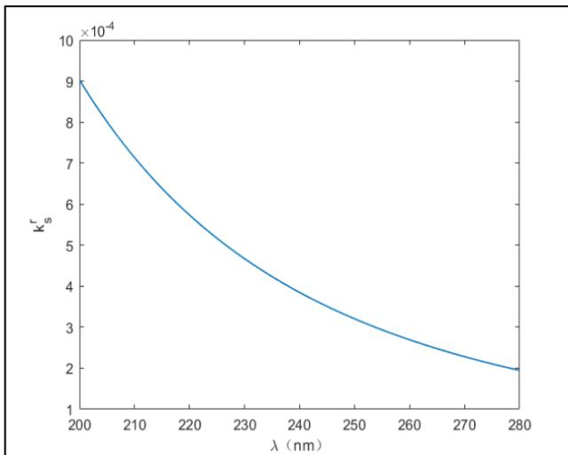
Fig 2: The Relationship between Rayleigh Scattering Coefficient and Wavelength
