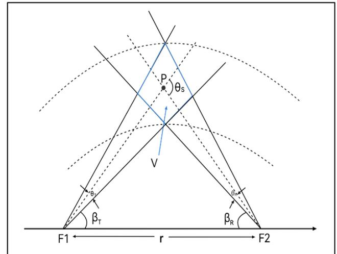
Fig 7: NLOS Ultraviolet Single Scattering Communication Link Diagram
