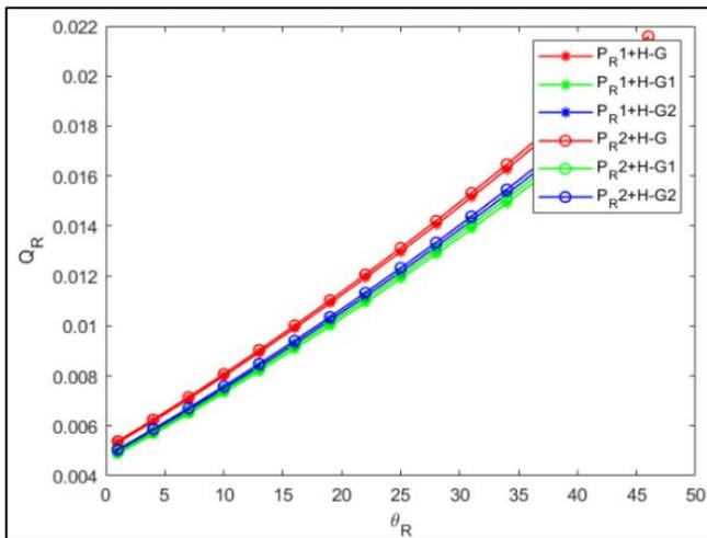
Fig 13: The Simulation Curve of Receiving Power Per Unit Area with the Change of Receiving Half Field Angle Under the Combination of Scattering Phase Function
