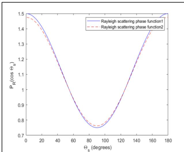
Fig 4: The Relationship between Rayleigh Scattering Phase Function and Scattering Angle
