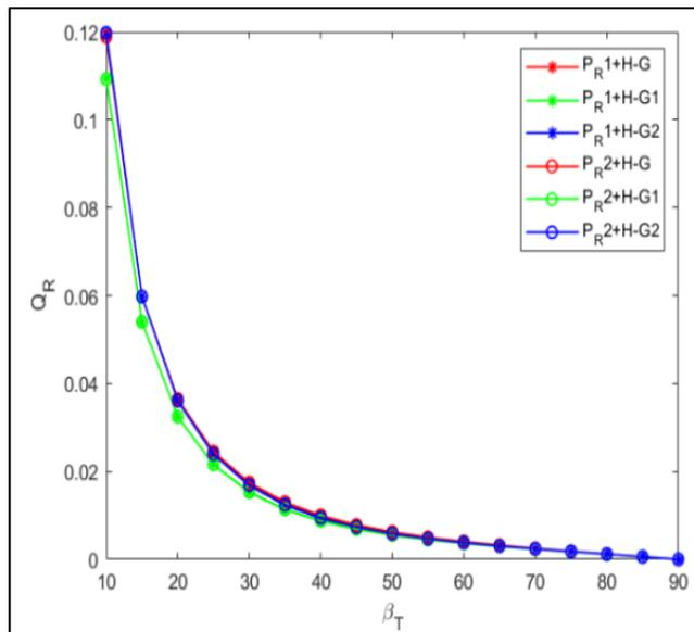
Fig 10: The Simulation Curve of the Received Power Per Unit Area with the Change of the Transmitting Elevation Angle Under Different Scattering Phase Function Combinations
