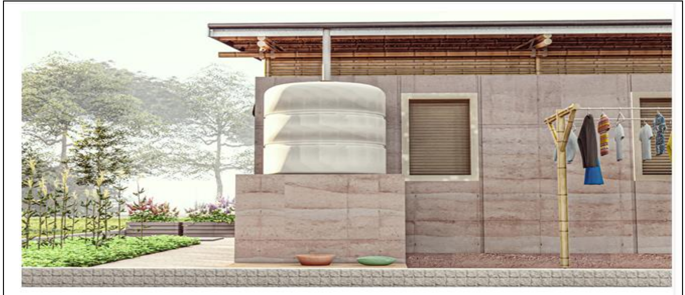
Fig 18: Illustration of Rainwater Harvesting System
