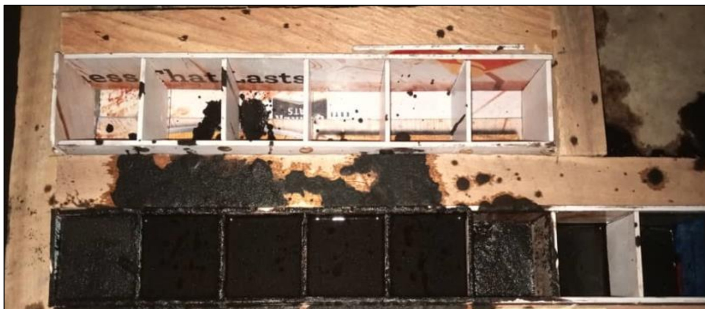
Fig 6 Process of Casting of Geopolymer Mortar in the Laboratory
