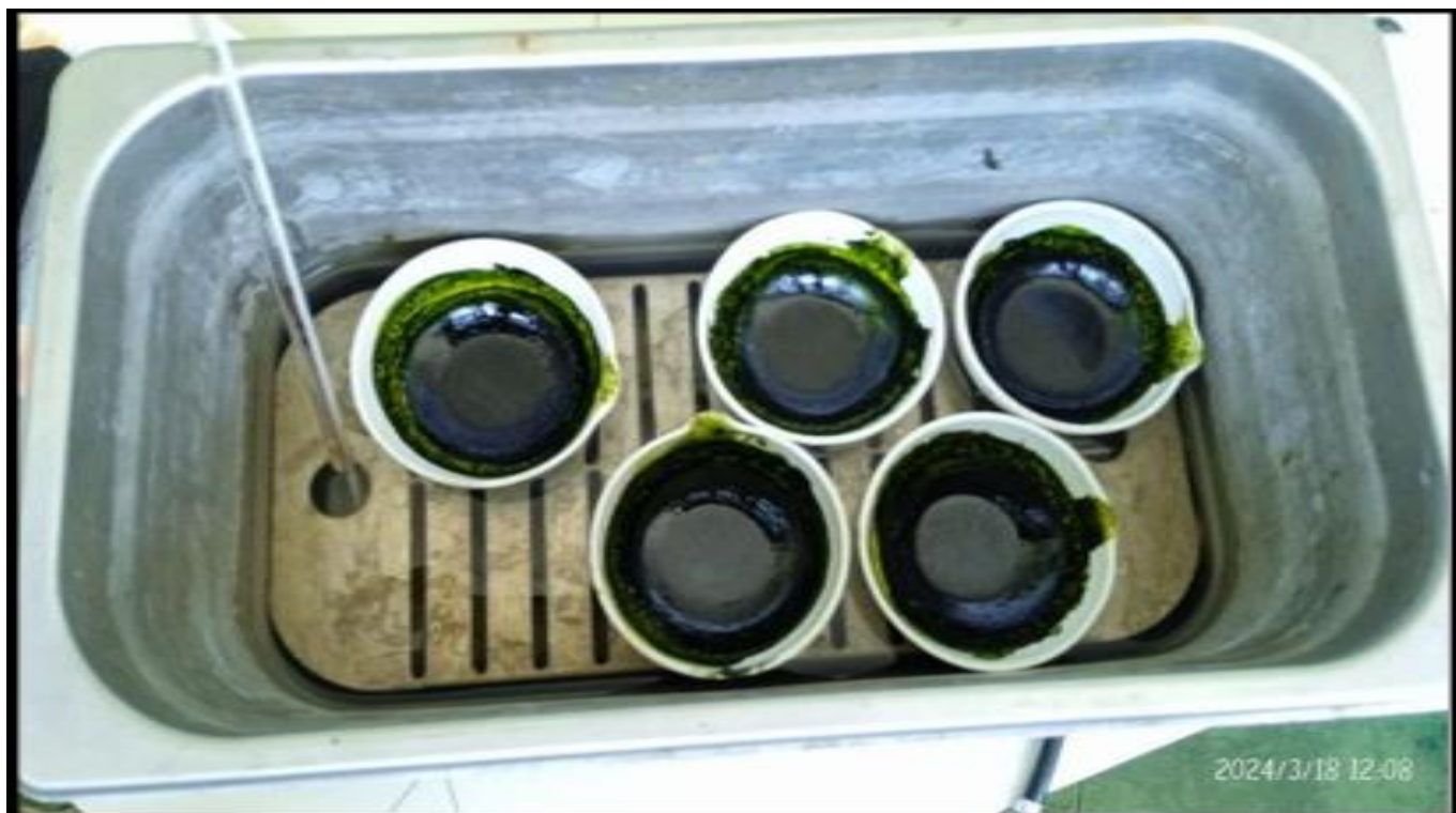
Fig 15: A Water Bath was Used on the Plant Material to Evaporate Further Impurities
