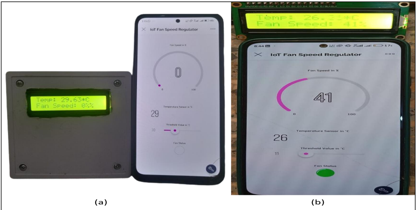
Fig 9 LCD and Blynk App Displaying the Temperature and Fan Speed (a) when below Threshold. (b) when above the Threshold.
