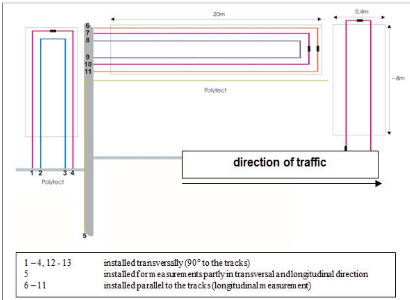
Fig 30: Position of the Sensors in the Test Side (Clemente Fuggini et al 2016)
