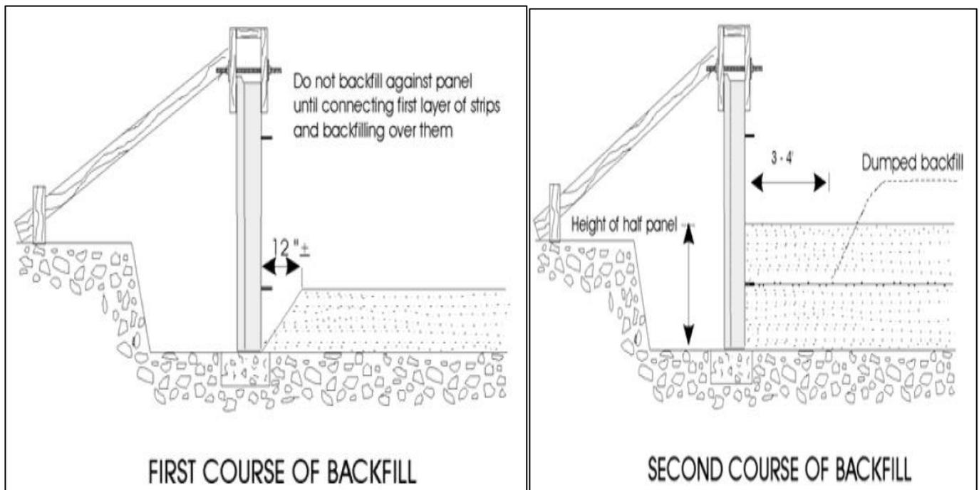
Fig 39: Placement of Backfill in Lifts to the Top of the Half Panels (Bailleul Guillaume and Laga Matthias 2017)
