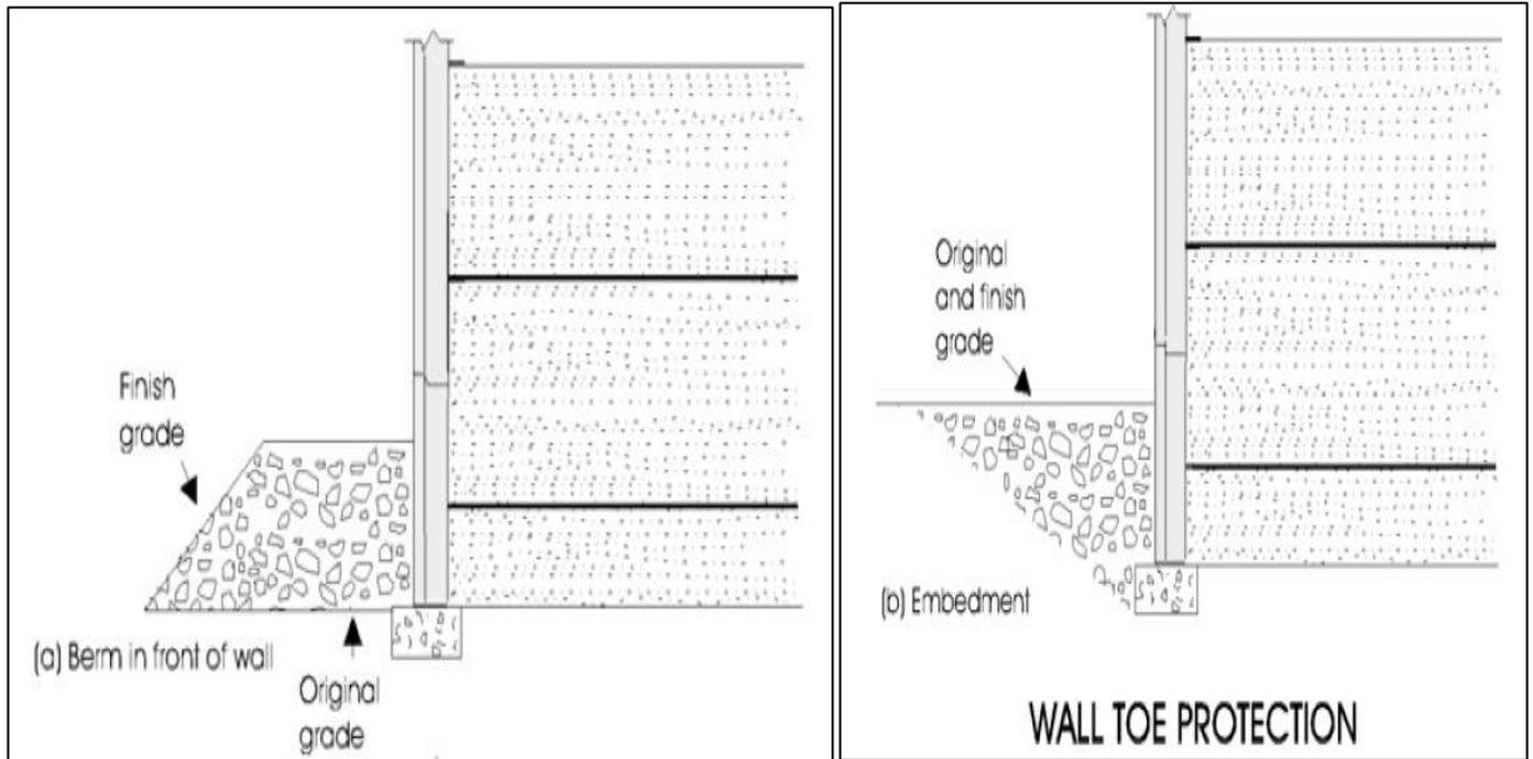
Fig 42: Placement and Compaction of an Embedment at the Lower Front Surface
