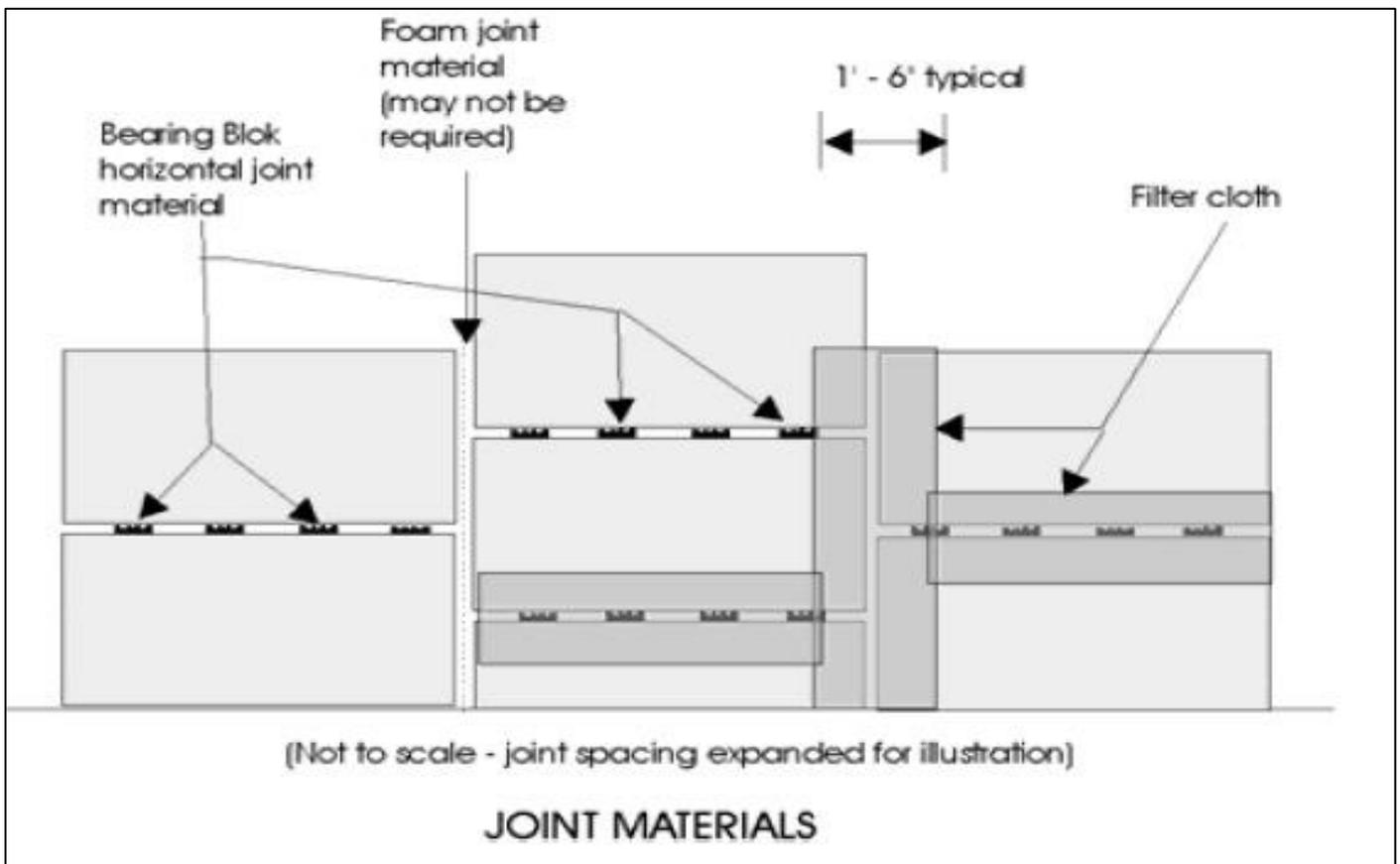
Fig 37: Use of Bearing to Avoid Concrete to Concrete Contact (Bailleul Guillaume and Laga Matthias 2017)
