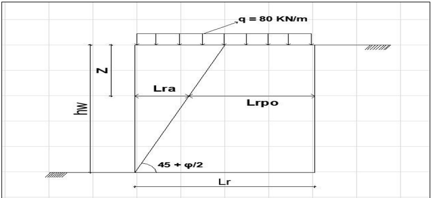
Fig 52: Illustration of the Reinforced Zone
