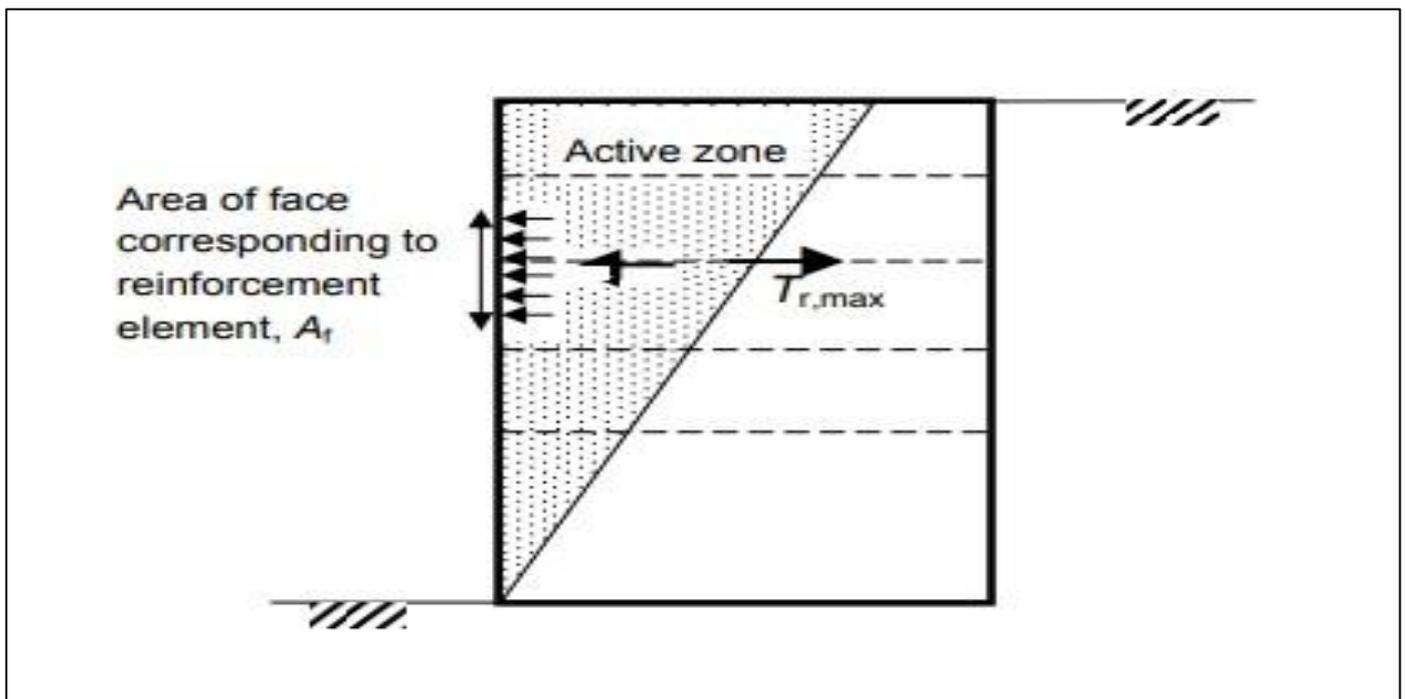
Fig 51: The Stresses Applied to the Facing and Reinforcing Element within the Active Wedge are Counteracted by the Maximum Tension  $T_{r,max}$  at the Back of the Wedge
