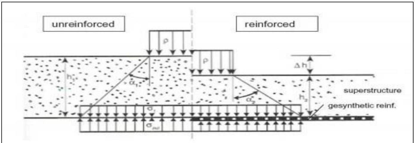
Fig 26: Use of Geotextiles for Soil Reinforcement (Clemente Fuggini et al 2016)
