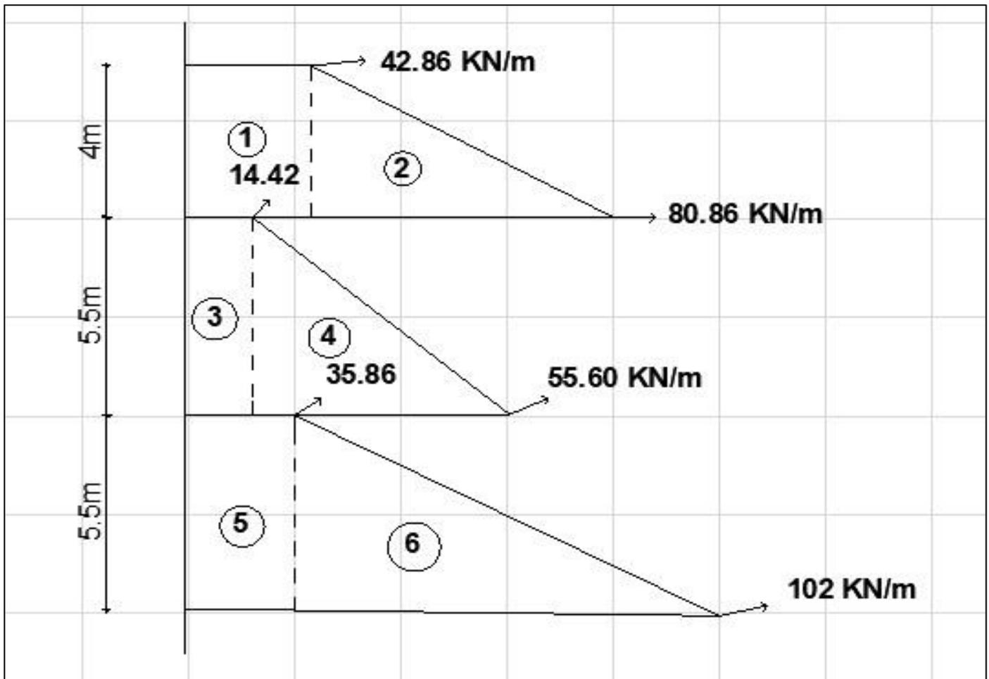
Fig 48: Active Pressure Distribution (APD) (Arch-Cad 2019)
