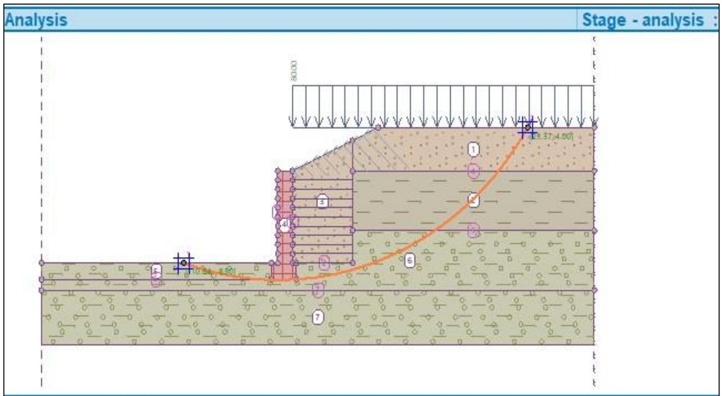
Fig 53: Model Description of the Wall (GEO 5, 2023.)
