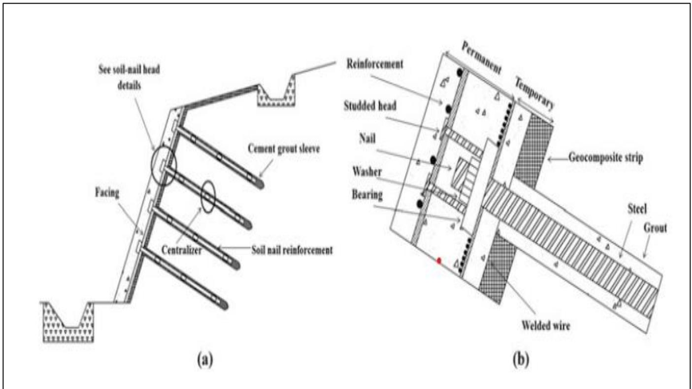
Fig 31: Schematic View of the Soil Nailed Slope (a) Cross Sectional View and (b) Details of Soil Nail Head (Mahesh Sharma, et al 2019)
