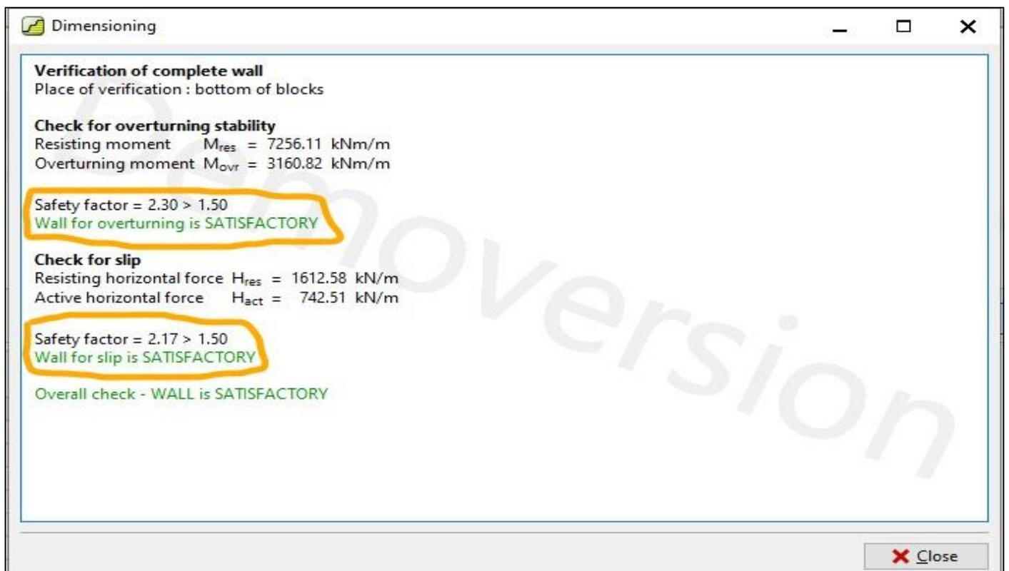
Fig 54: Overturning and Sliding Stability Result (GEO 5, 2023.)
