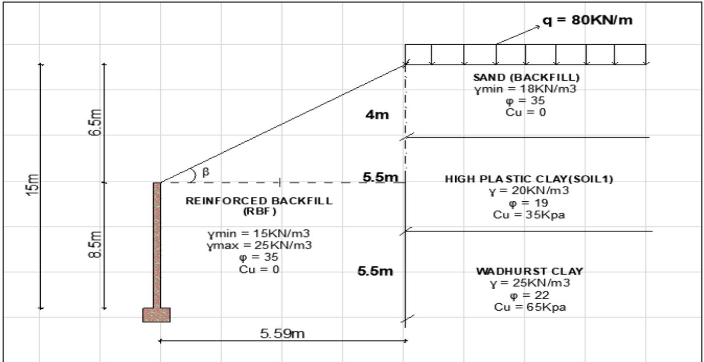
Fig 47: Section of the Wall to be Considered (Arch-Cad 2019)
