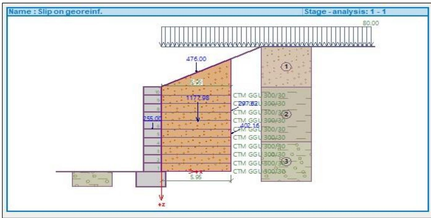
Fig 61: Geo-Reinforcement Model (GEO 5, 2023.)
