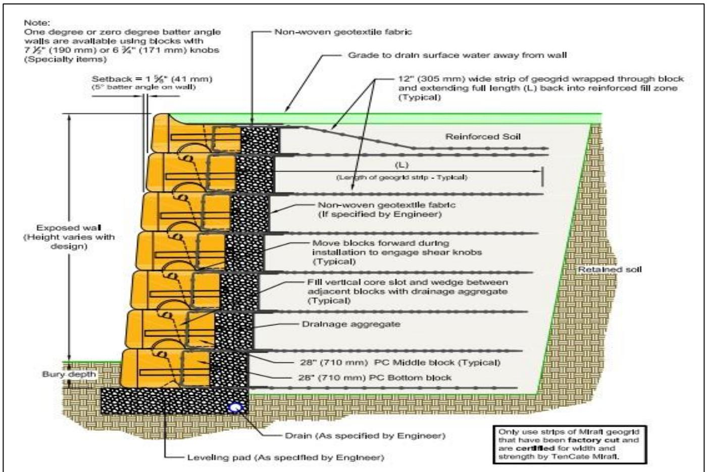
Fig 8: Typical Mechanical Stabilize Earth Wall Section (Redi-Rock 2020)
