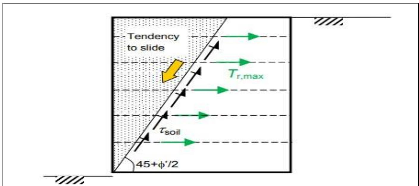
Fig 50: The Active Wedge Leads to Active Earth Pressure by Trying to Slide Downward and Outward, but this is Counteracted by Soil Shearing and the Tension in Reinforcing Elements that Anchor it
