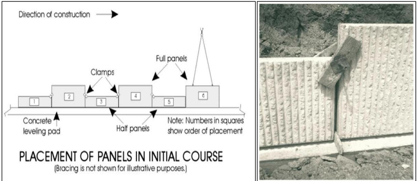
Fig 36: Positioning the Panels in the Starting Row onto the Concrete Levelling Pad.(Bailleul Guillaume and Laga Matthias 2017)
