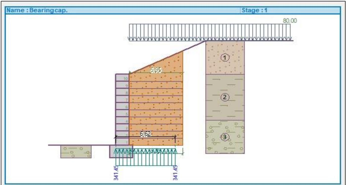
Fig 57: Bearing capacity model (GEO 5, 2023.)
