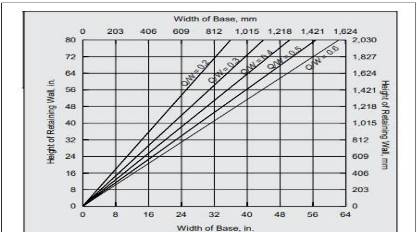
Fig 3: Relationship of Gravity Retaining Wall Height to Width at Base (NCMA 2023)
