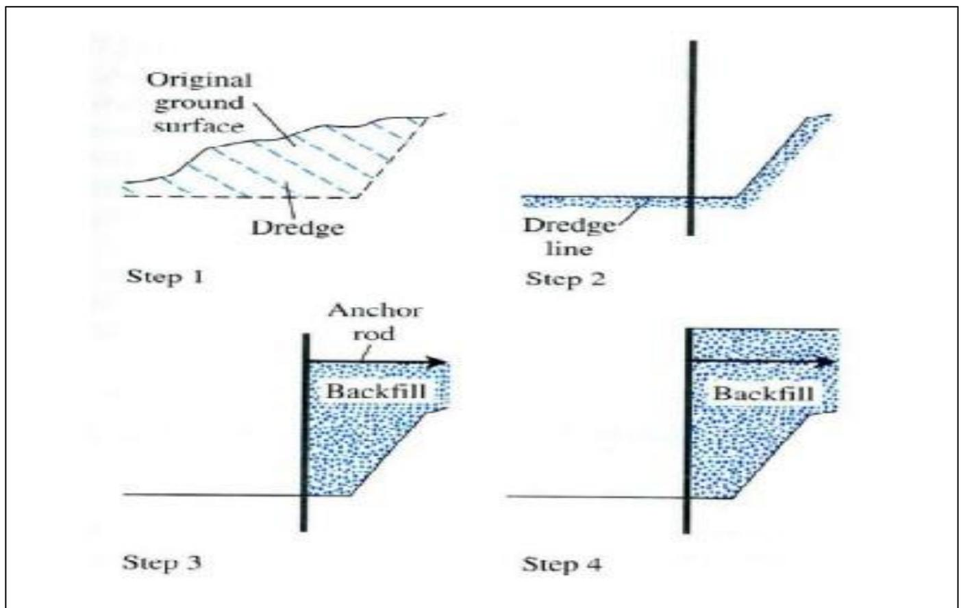
Fig 18: Construction Sequence for a Back-Filled Structure (Ahmed H.A 2017)
