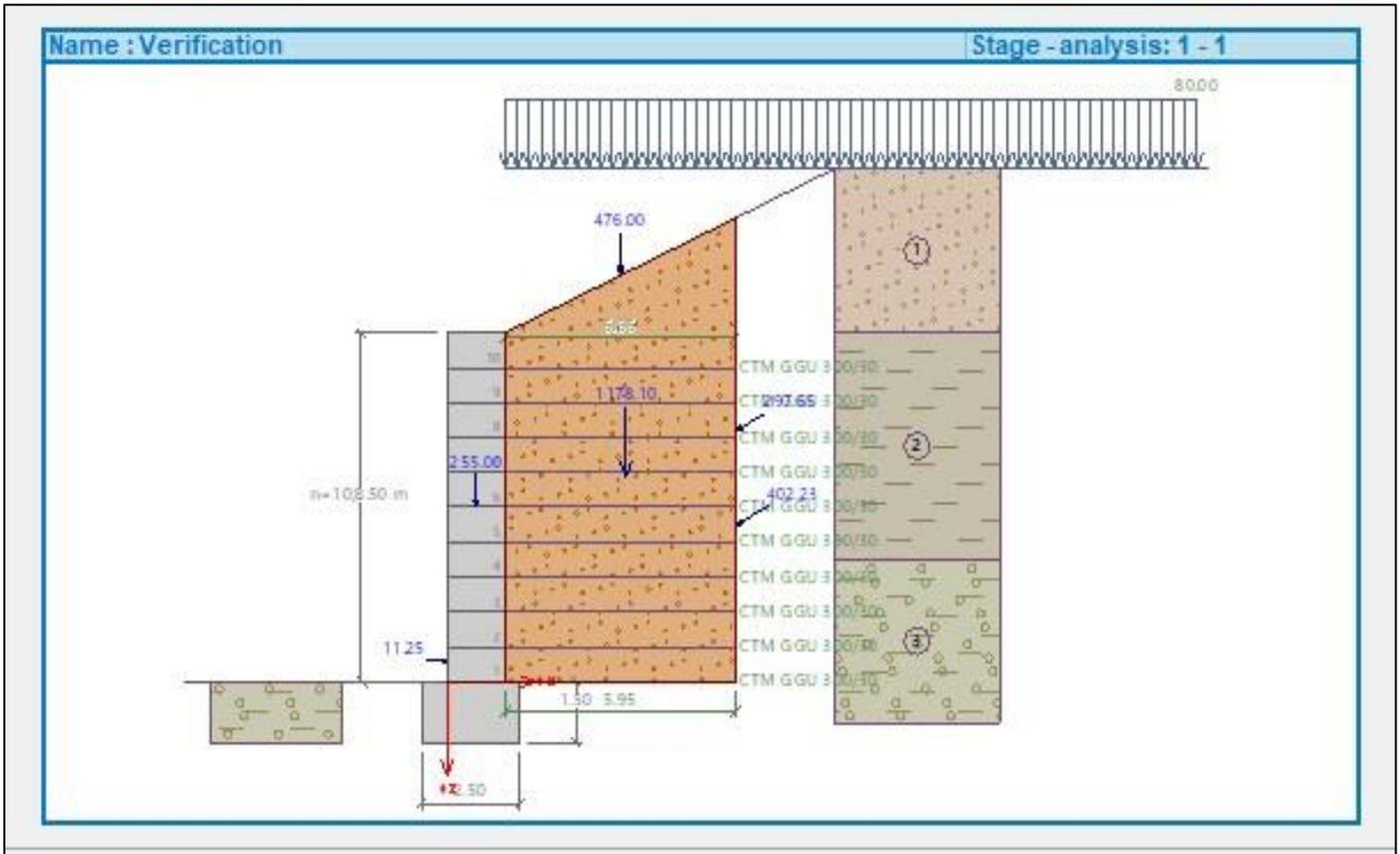
Fig 55: Overturning and Sliding Stability Model (GEO 5, 2023.)
