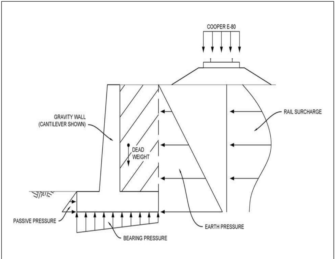
Fig 20: Gravity Retaining Wall Schematic Bryan Duevel et al (2014)
