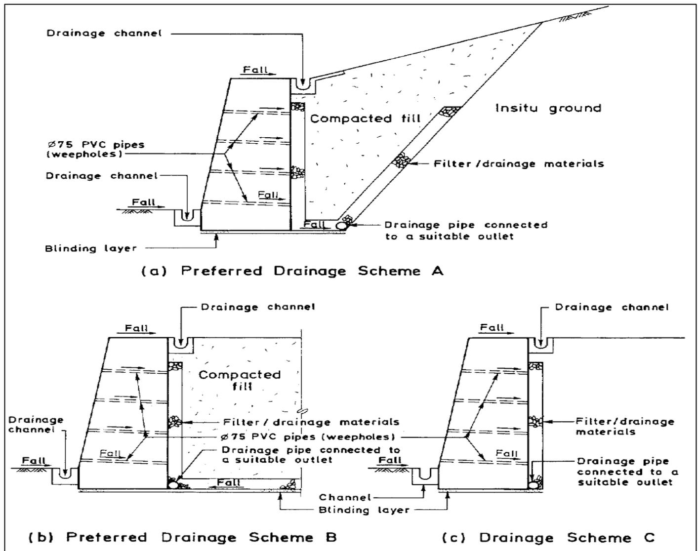
Fig 4: Drainage Schemes for Gravity Retaining Walls (geotechnical Engineering Office, (1993)
