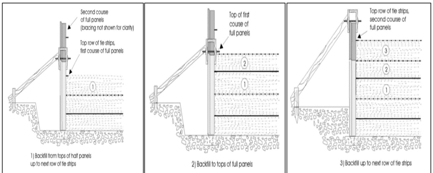
Fig 41: Adding Backfill in Layers Until It Reaches the Level of the Tie Strip
