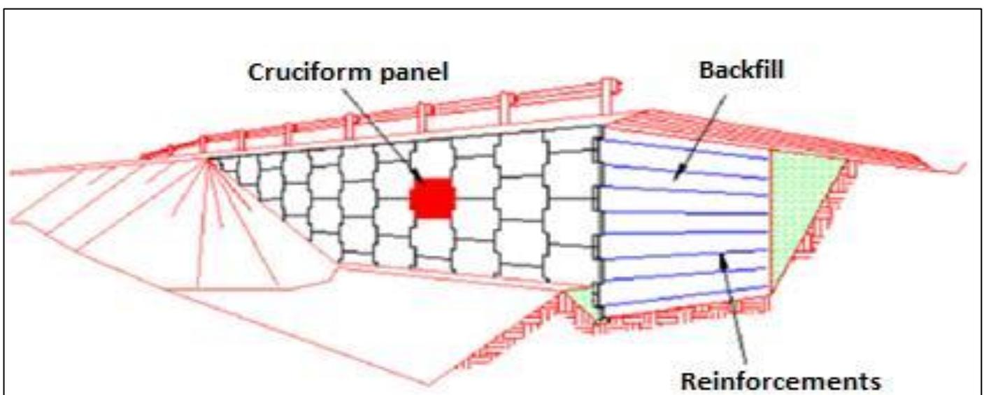
Fig 5: MSE Walls System (Alhajj Chehade et al., 2019)
