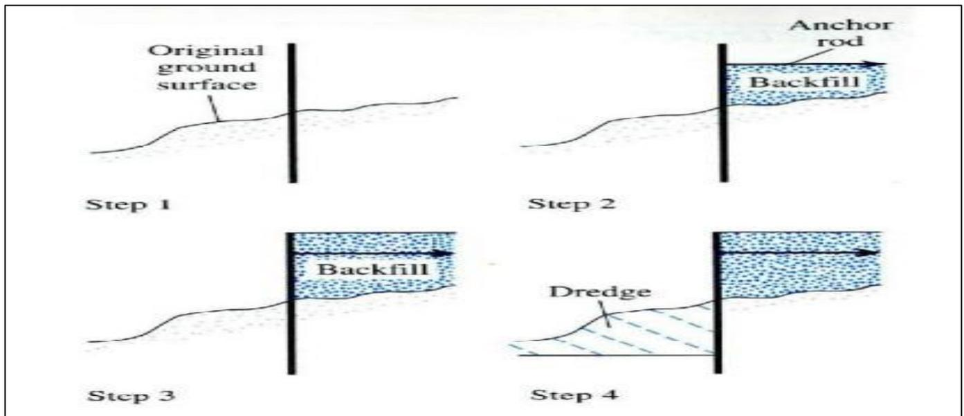
Fig 19: Construction Sequence for a Dredged Structure (Ahmed H.A 2017)
