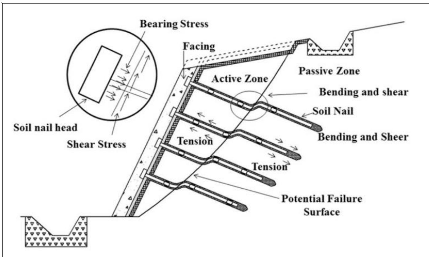
Fig 33: Failure Mechanism of Soil Nail System (Mahesh Sharma, et al 2019)
