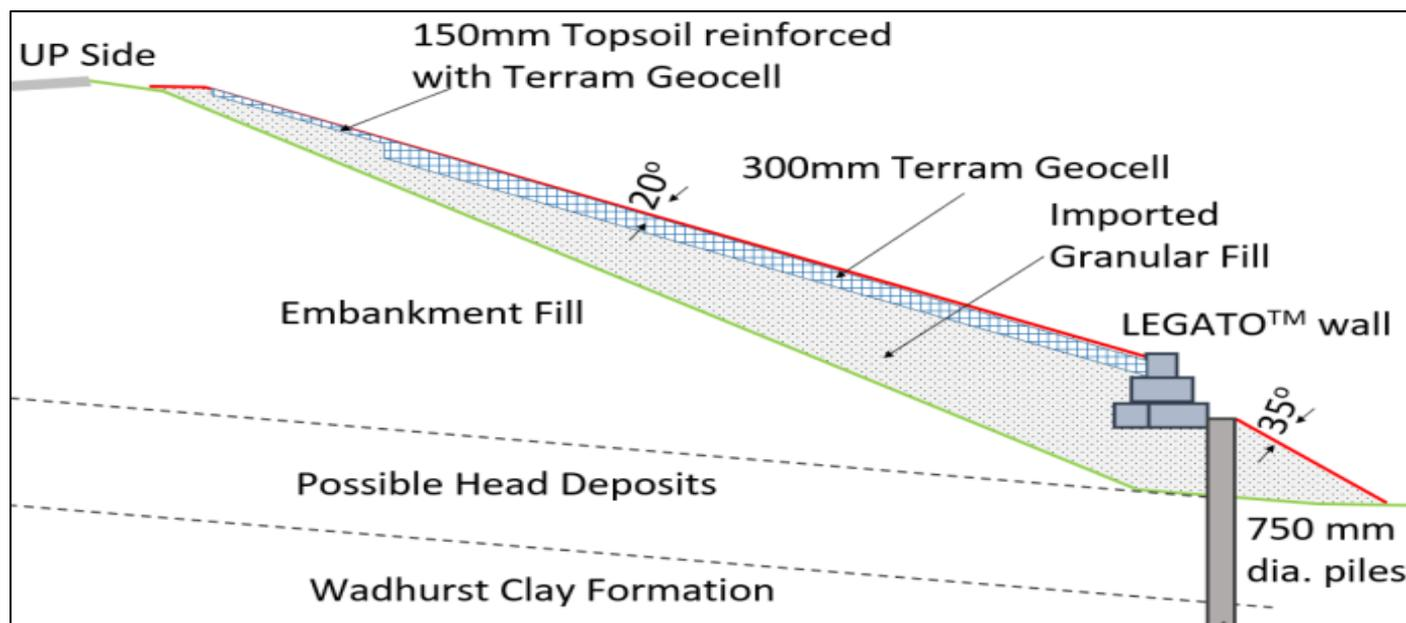
Fig 34: Proposed Case Study Design of the Balcombe Embankment (B. Burcin Avar et al 2023)
