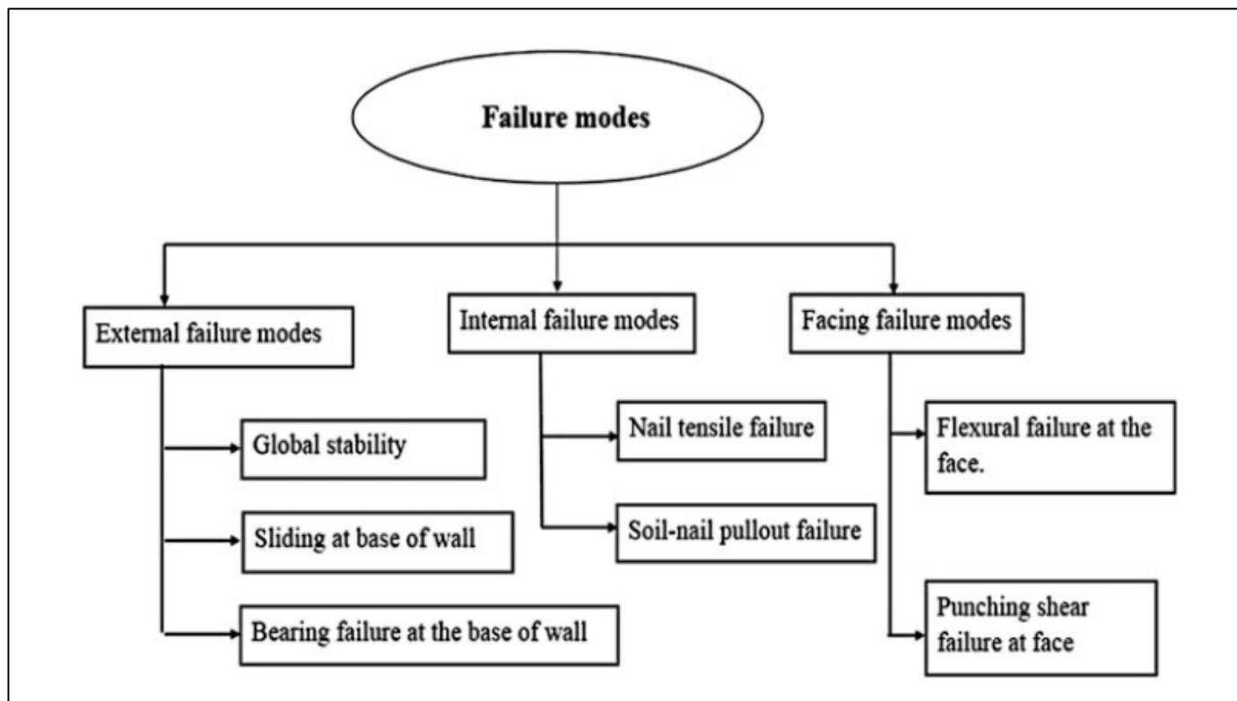
Fig 32: Failure Modes of Soil Nailing System
