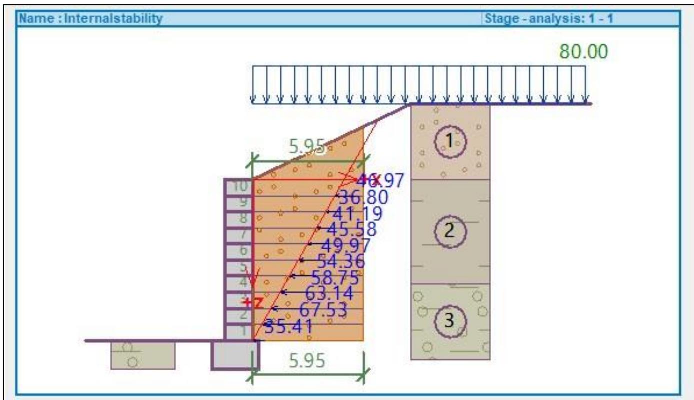
Fig 59: Tensile Strength and Pullout Resistance Model (GEO 5, 2023.)
