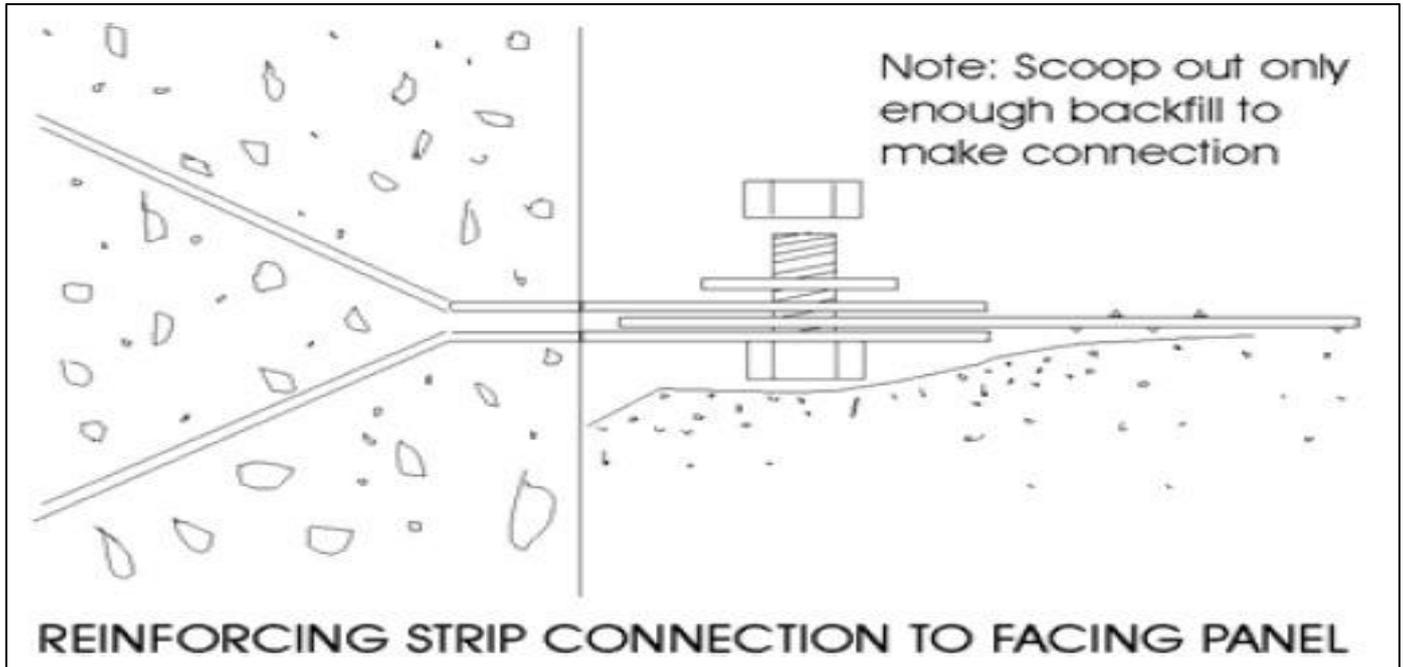
Fig 38: Connection of Reinforcing Strips to the Facing Panels (Bailleul Guillaume and Laga Matthias 2017)
