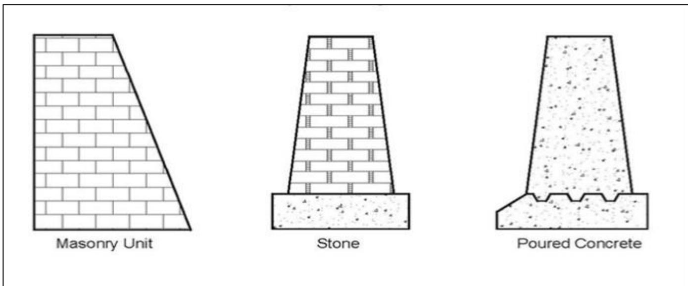
Fig 1: Gravity Retaining Wall from Masonry Unit, Stone or Mass in-Situ Concrete (Tensar Website )
