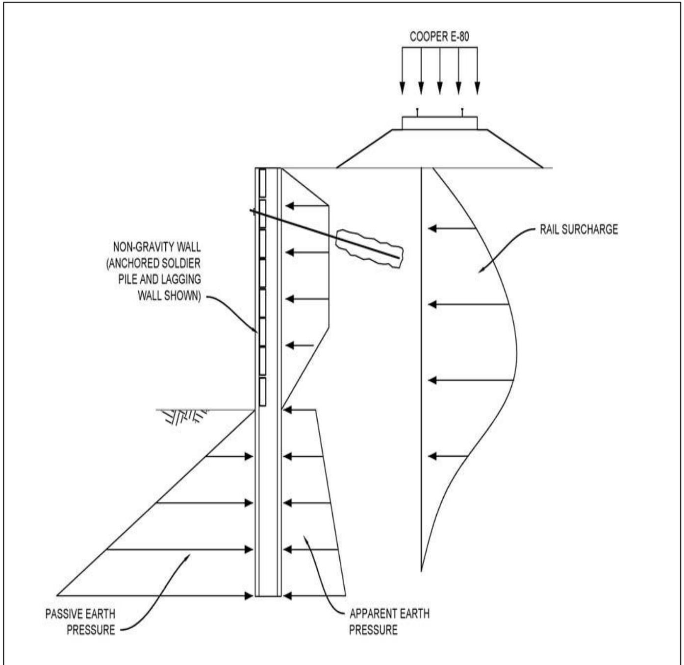
Fig 21: Non-Gravity Retaining Wall Schematic Bryan Duevel et al (2014)
