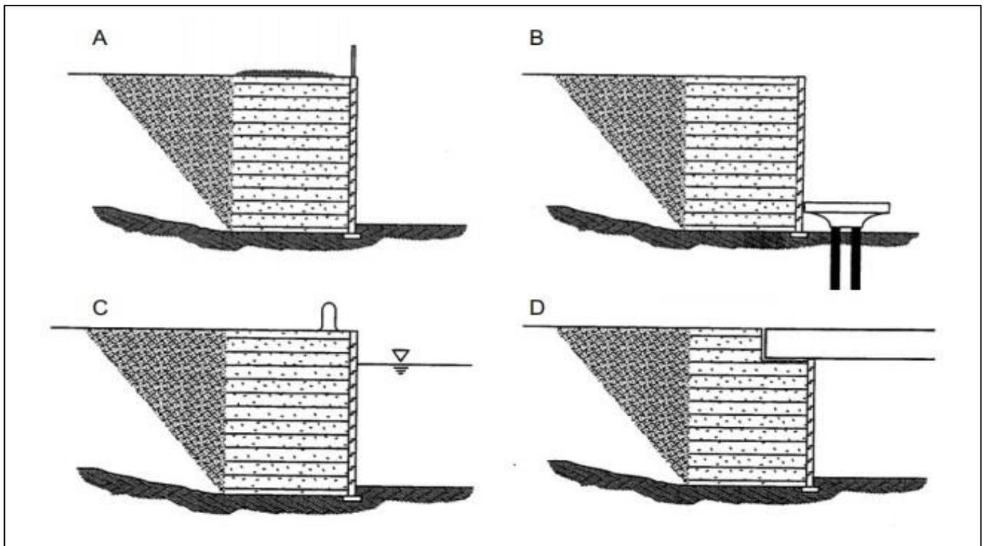
Fig 14: MSE Wall Applications (A) Retaining Wall; (B) Access Ramp; (C) Waterfront Structure; and (D) Rail Infrastructure / Bridge Abutment [6] (Bailleul Guillaume and Laga Matthias (2017)
