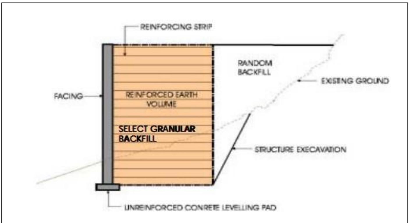
Fig 7: Component of Mechanical Stabilized Earth Walls (Keith Brabant, 2001)
