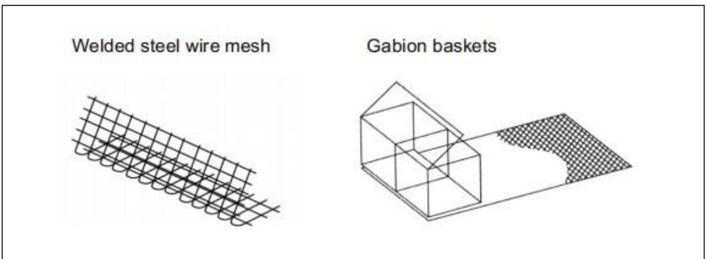
Fig 13: Mechanical Stabilized Earth Steel Facing Unit (Bailleul Guillaume and Laga Matthias, (2017)
