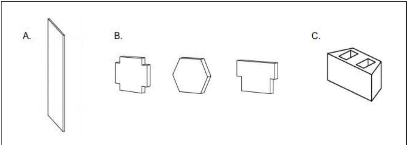
Fig 12: A. Full Height Panels – B. Partial Height Panels – C. Segmental Blocks (Bailleul Guillaume and Laga Matthias, 2017)
