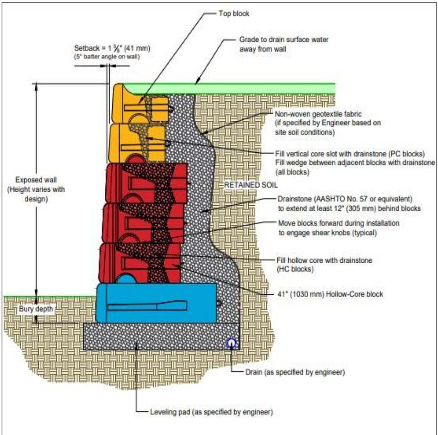
Fig 2: Typical Gravity Wall Detail with Hollow-Core Blocks (Redi-Rock 2020)
