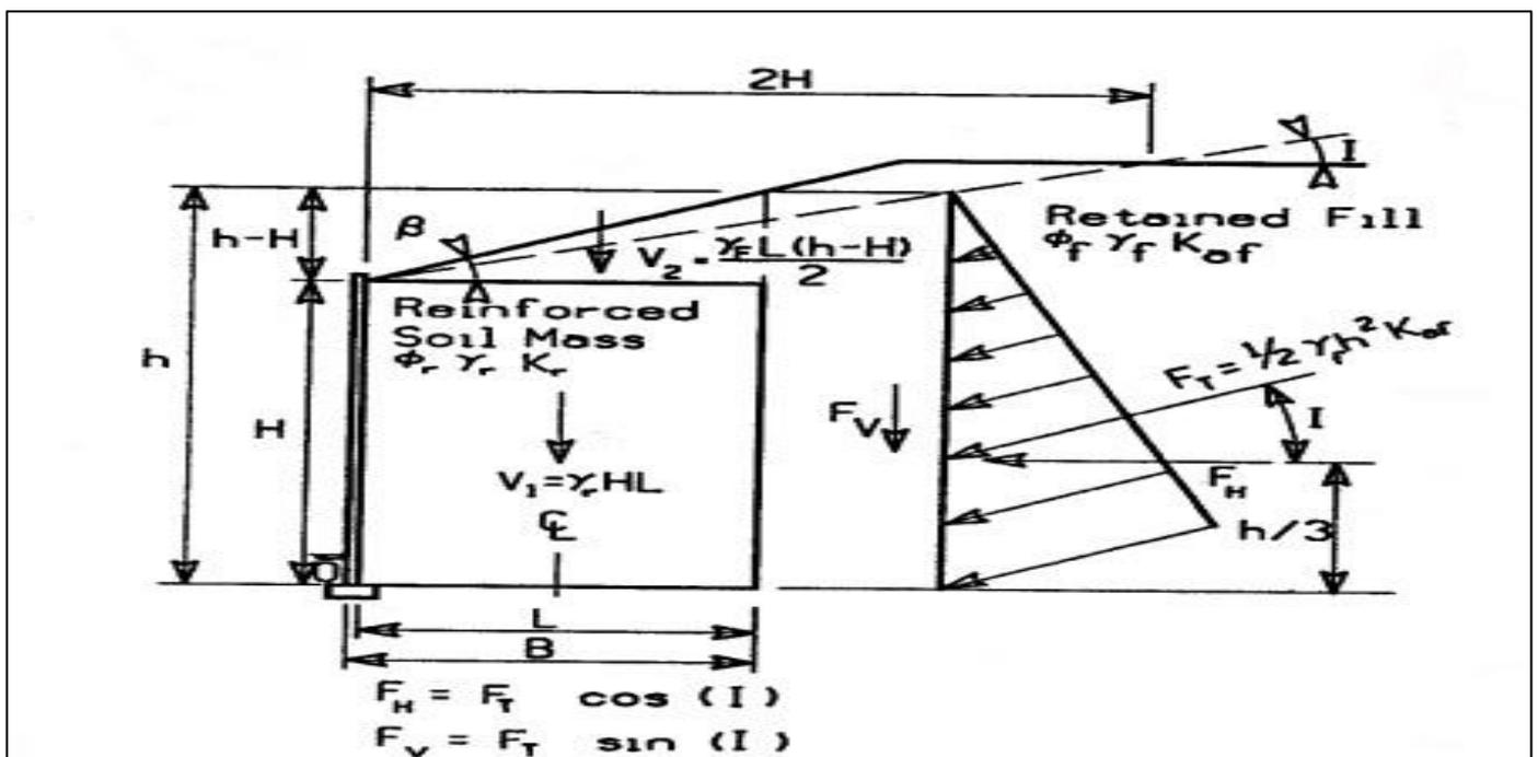
Fig 46: Sloping Back-Slope Case of the (RSW)
