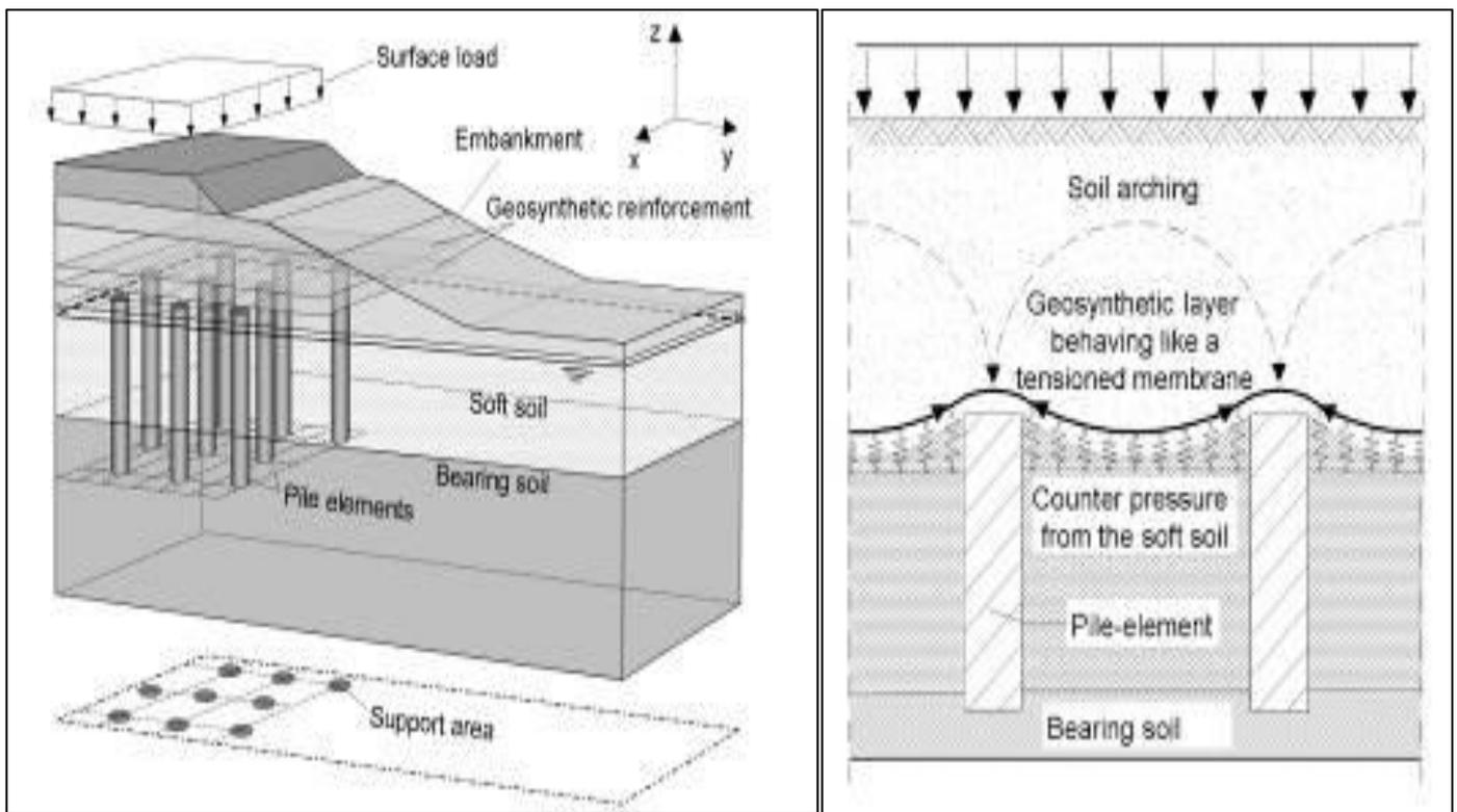
Fig 27: Geosynthetic-Reinforced and Pile-Supported Embankment (Clemente Fuggini et al 2016)
