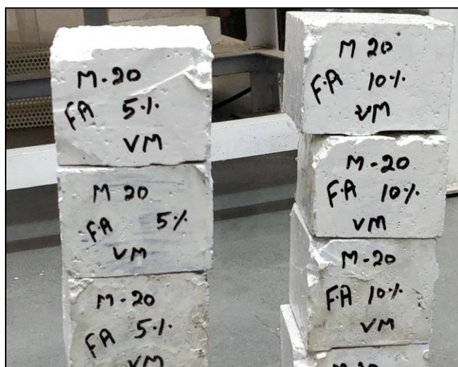
Fig. 1. Specimen Prepared after Cutting and Coated with Epoxy.
