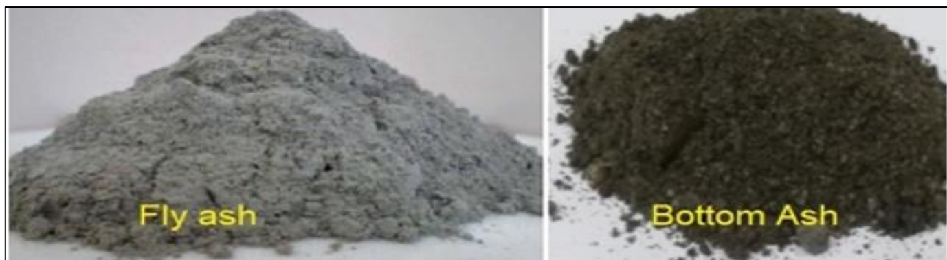
Fig 7: Shows Real-Life Images of Fly Ash and Bottom Ash Compared to One Another. Fly Ash (Left) is the Finer Powder Made from Incineration that Goes into the Air and has Higher Concentrations of Heavy Metals. Bottom Ash (right) is the Coarser Ash Left at the Bottom of an Incinerator with Lower Concentrations of Heavy Metals. (What Is Ashcrete?, 2022)
