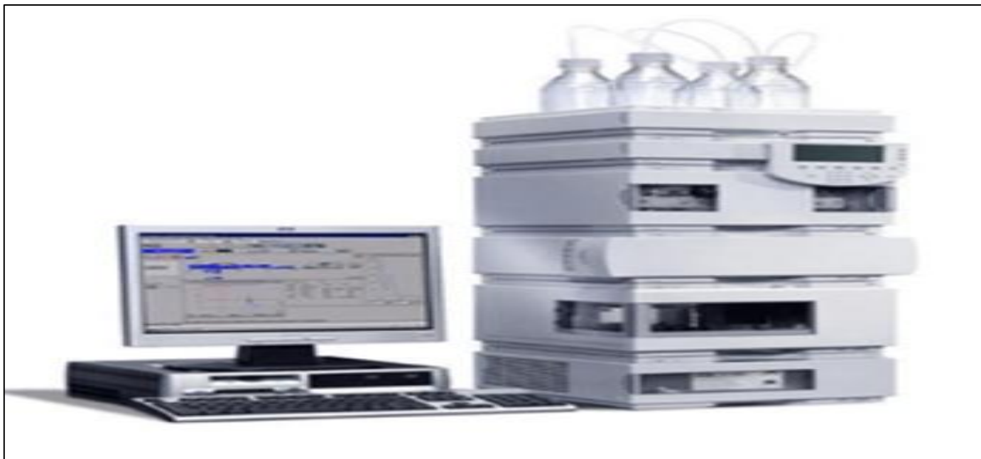
Fig 27: A method used by Eurofins Lab to Collect the Data Needed, High-Performance Liquid Chromatography, and Liquid Chromatography-Mass Spectrometry. Inductively Coupled Plasma Atomic Emission Spectroscopy was also Used
