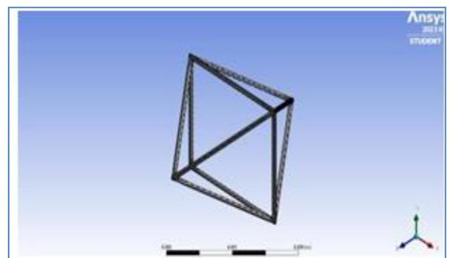
Fig. 6: Meshing of an Octahedron cell
