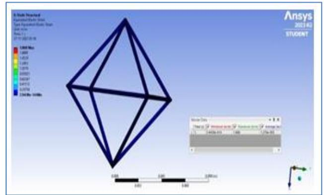
Fig. 8: Static Structural Analysis Done for Equivalent Strain on the Cell
