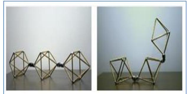
Fig. 1: Representation of Morphing Structure using Octahedron Cells
