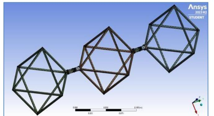
Fig. 5: Meshing of the Octahedral Structure done on ANSYS.
