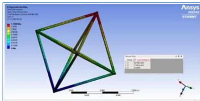
Fig. 10: Static Structural Analysis Done for Total Deformation Under Buckling Effect on the Cell
