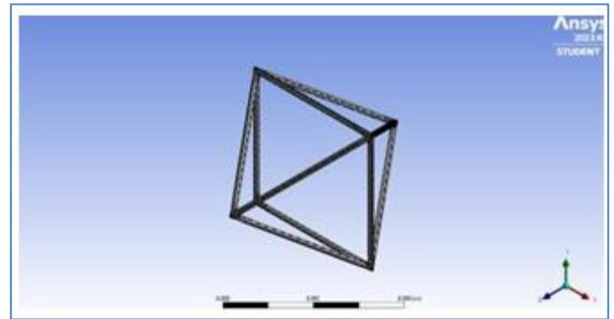
Fig. 4: Figure Represents a Successful mesh of an Octahedron Cell
