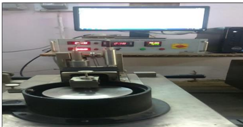
Fig.4 Setup of Pin on-Disc wear test [16]
