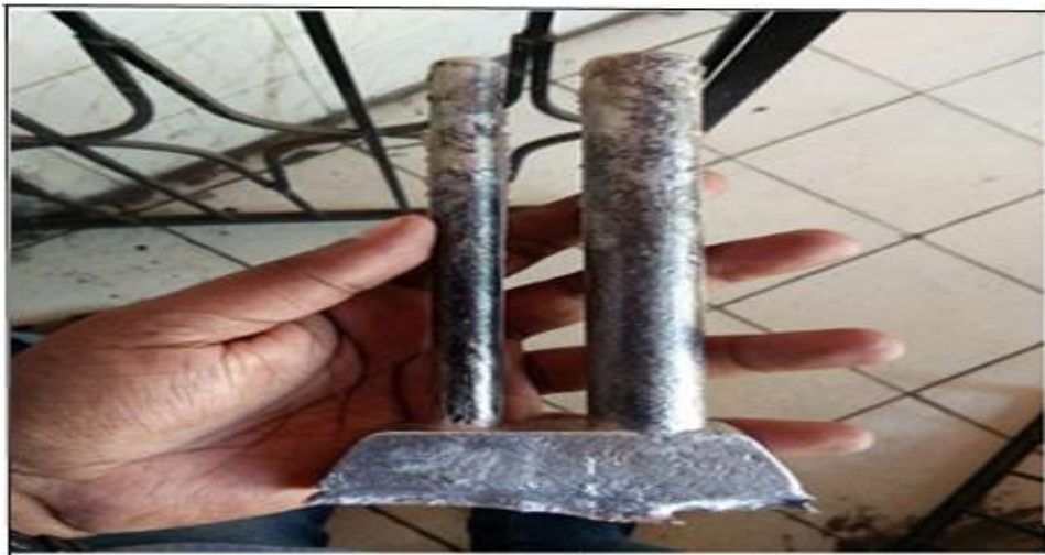
Fig 2. Sample of AMC Having 4% Al 2 O 3 Casted at 820°C
