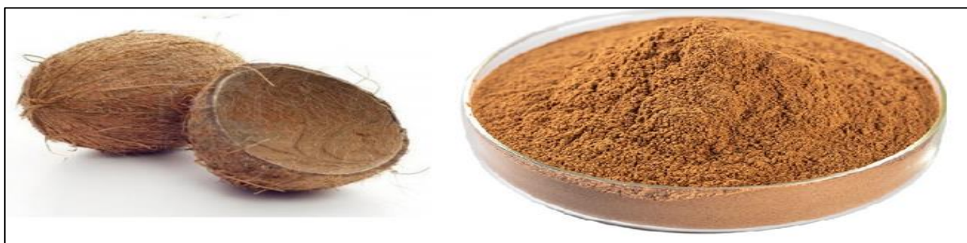
Fig 2: Coconut Shell and Coconut Shell Powder used as Adsorbent
