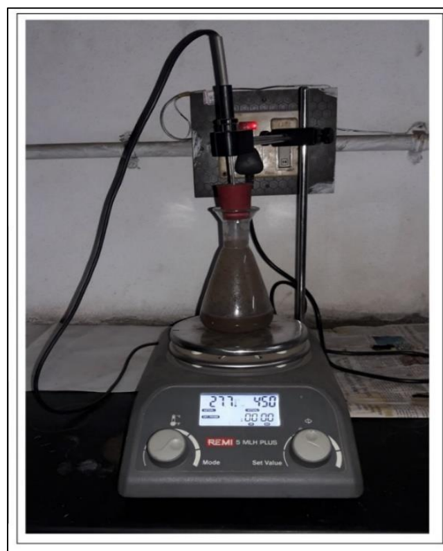
Fig 12: Equipment having Heater with Magnetic Stirrer Arrangement
