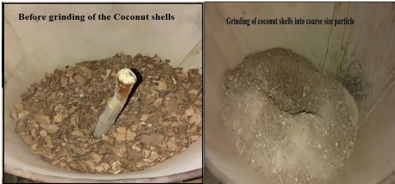
Fig 6: Preparation of Adsorbent (Coconut Shell Powder)
