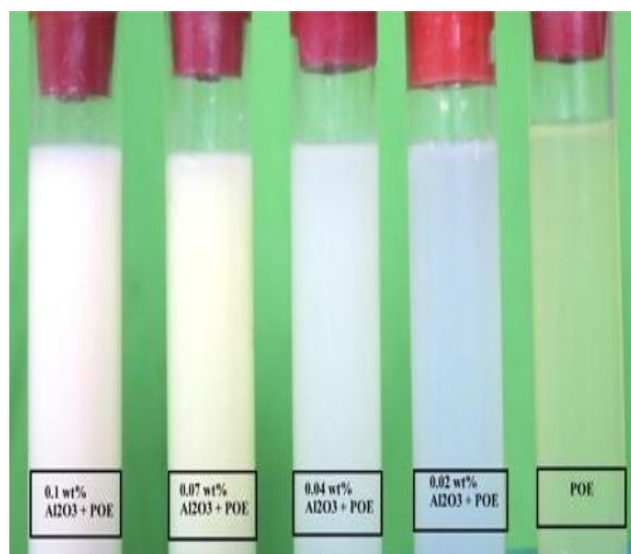
Fig 7: Different Concentration of AL2O3 Nanofluid with POE Oil
