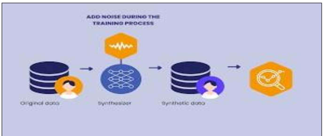
Fig 16: Here We Can See How Some Noise is Added to the Original Dataset to Form a New Dataset that is More Robust Against Inversion Attacks
