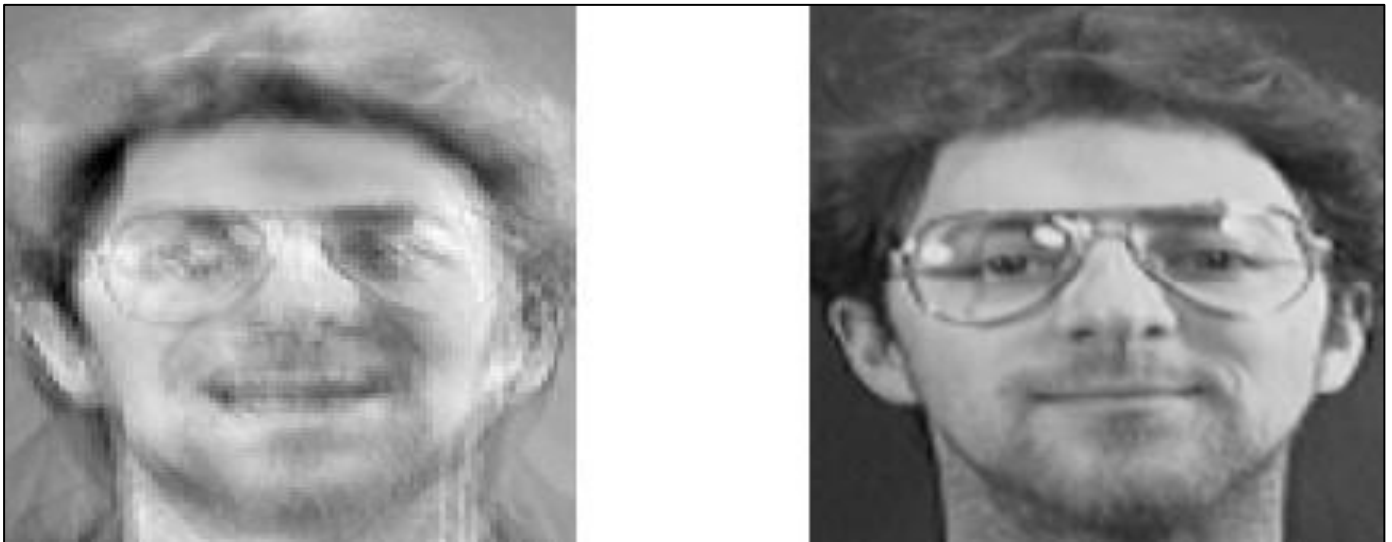
Fig 9: An Image Recovered Using a New Model Inversion Attack (Left) and a Training Set Image of the Victim (Right). The Attacker is Given Only the Person's Name and Access to a Facial Recognition System that Returns a Class Confidence Score.
