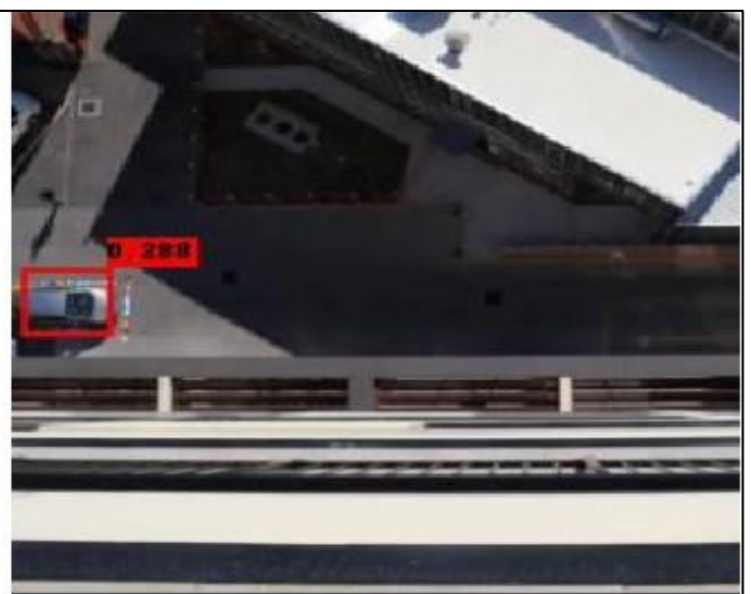
(f) The car in (d) imaged with a physical off-car patch; the objectness score reduced to 0.288.
