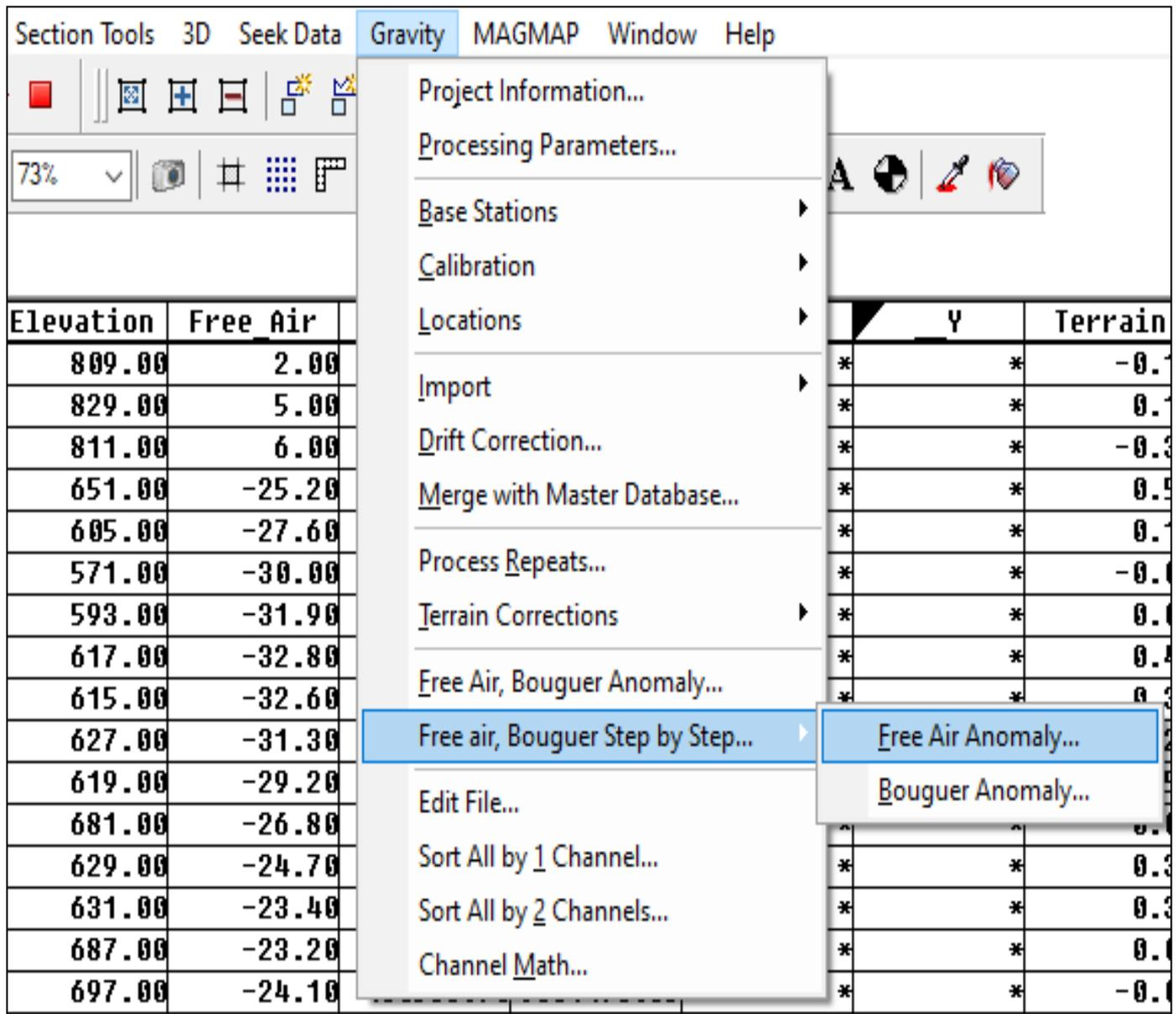
Fig 3: Tabs for Applying the Free-Air and Bouguer Corrections with the “GX - Gravity” Extension of the Oasis Montaj Software
