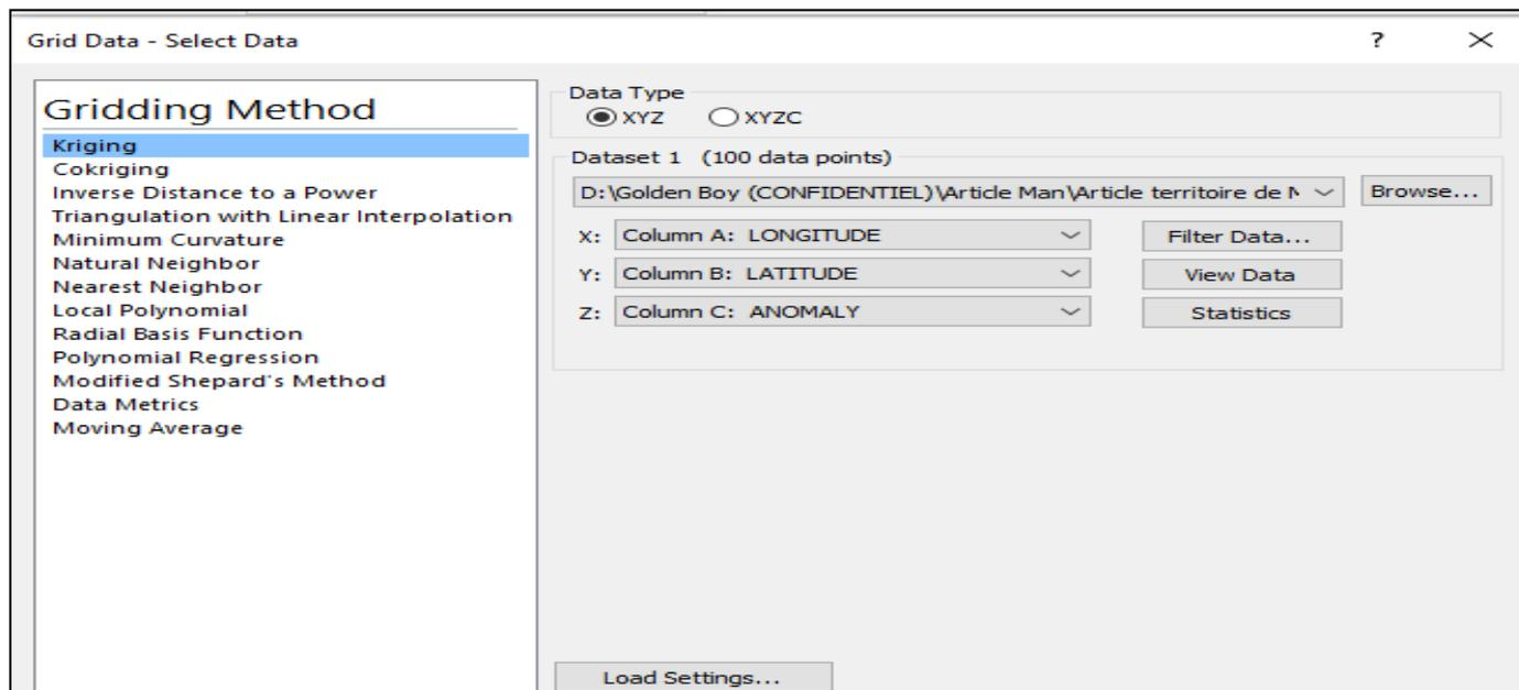
Fig 4: Window for Spatial Interpolation of Gravity Data from Golden Surfer Software
