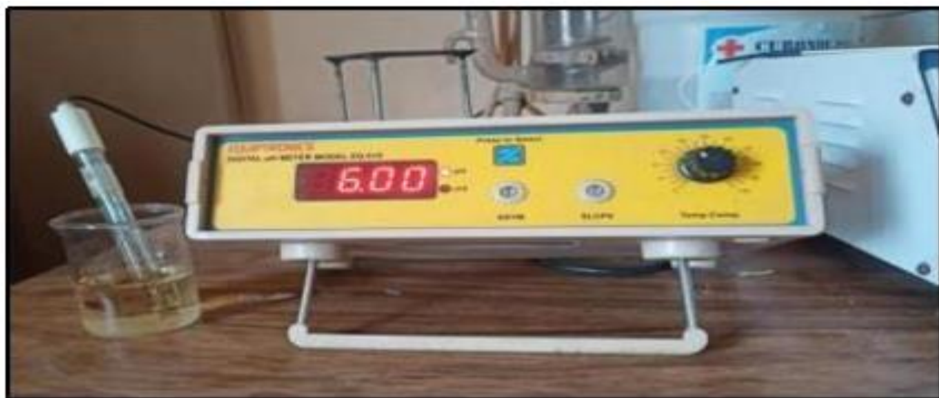
Fig 8: Digital pH Meter
