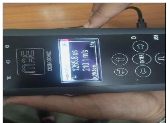
Fig. 4: Readings on Ultrasonic Pulse Velocity Meter
