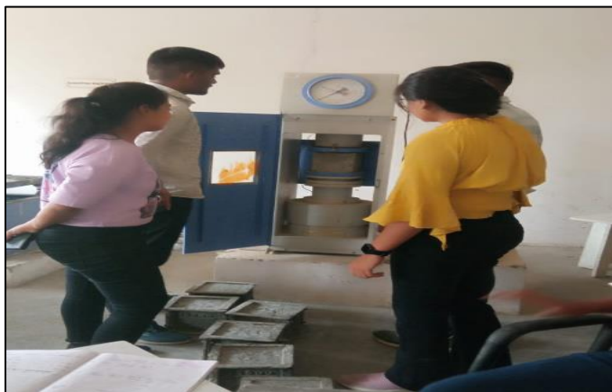
Fig 3: Testing Compressive Strength of Cubes
