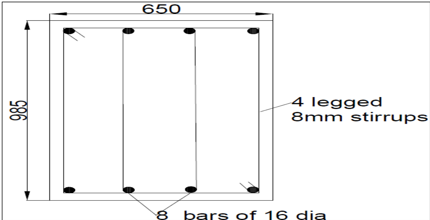
Fig 28: Ring Girder Detailing in Manual Design
