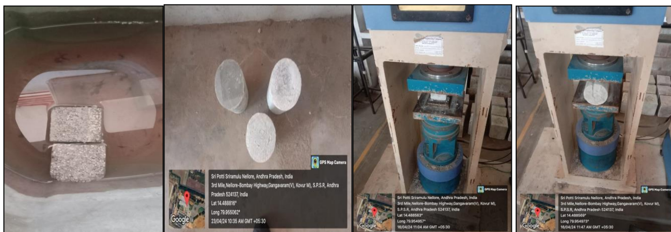
Fig 3: Destructive Tests of Floating concrete
