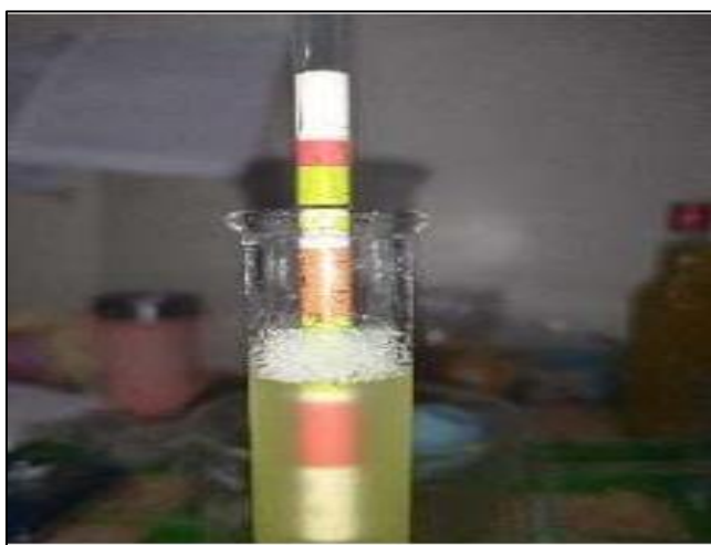
Fig 102: Trial 5 Sugar Adjustment: 20% Sucrose Level on Hydrometer
