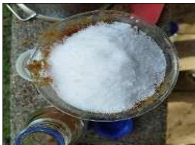
Fig 34: Trial 1 Fermentation Process: Adding of Sodium Hydroxide
