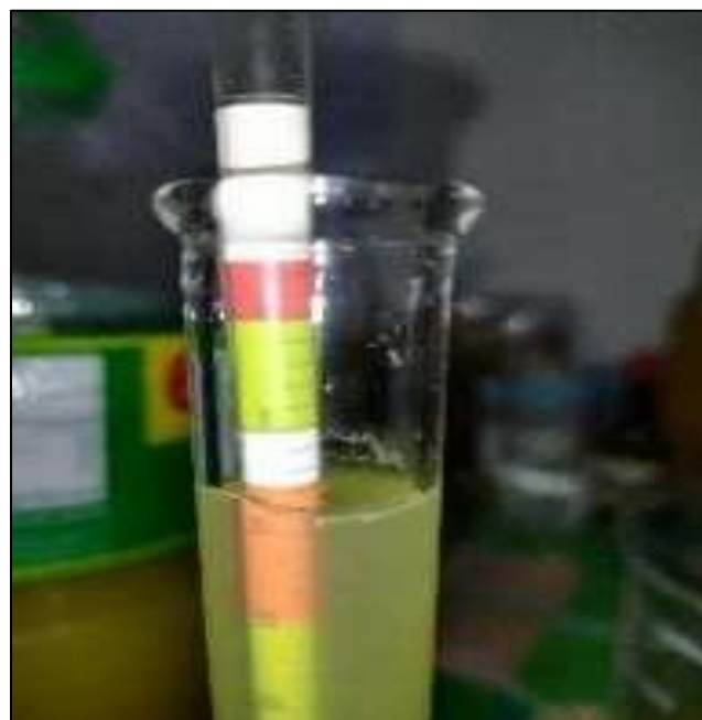
Fig 99: Trial 5 Sugar Adjustment: 9% Sucrose Level on Hydrometer
