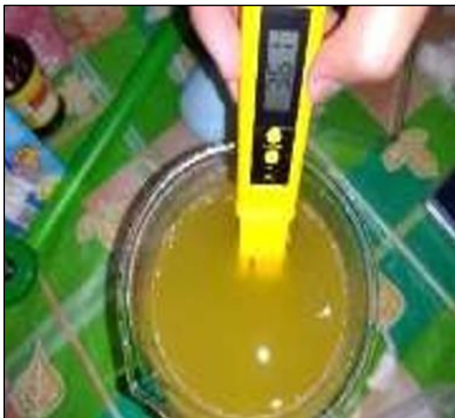
Fig 122: Trial 6 pH Adjustment: 3.61 pH Level on a pH Meter
