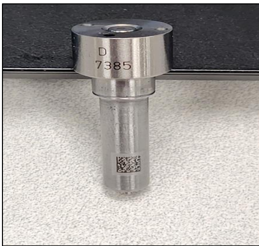
Fig 2 Nozzle after Recalim Process
