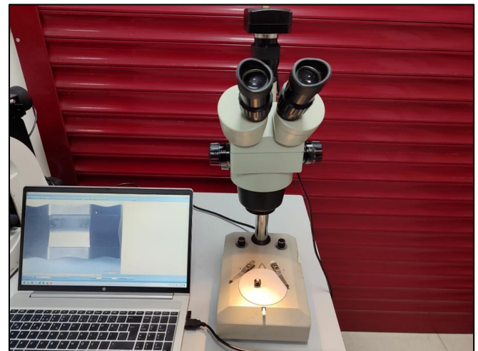
Fig 7 Examining the Cutting tip with a Microscope
