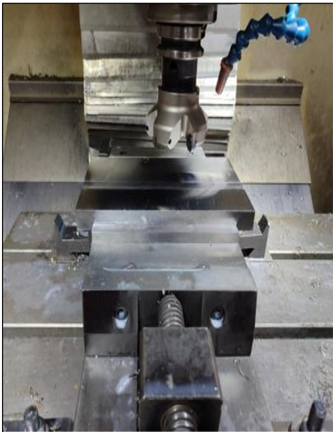
Fig 5 Test Sample Surface Milling Process
