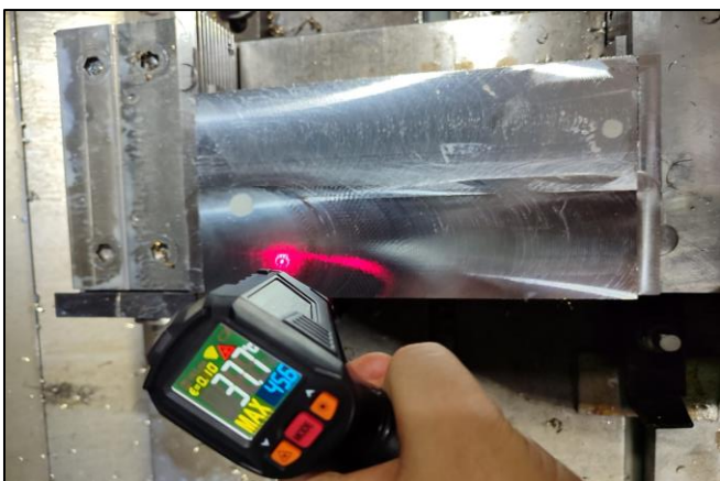
Fig 6 Surface Temperature Measurement with Heat Detector
