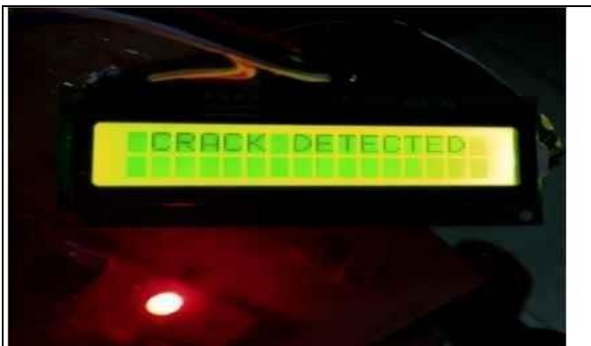
Fig 13: LCD Displaying Crack Detected Message
