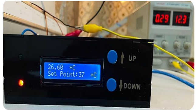
Fig 8: The Incubator Heater Operating
