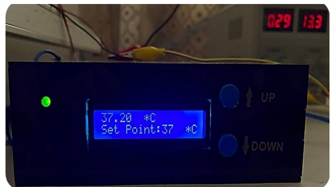
Fig 9: Green Light Indicates the Required Temperature is Reached
