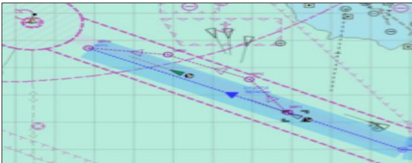
Fig 14: Example of AI-Generated Ship Trajectory, Dynamic Safety Domain and Safe Route for Ships to Diverge
