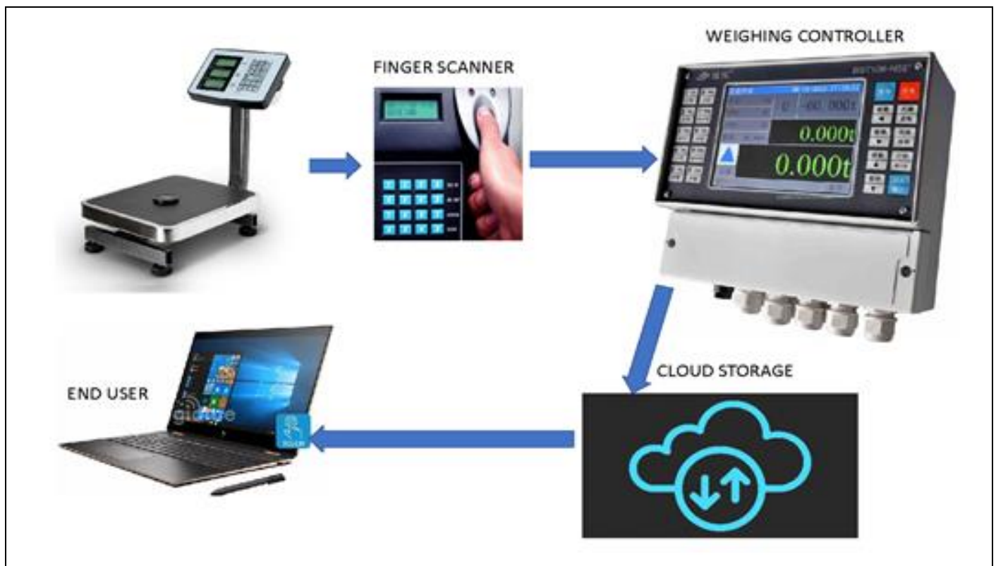
Fig 1(A): Schematic Diagram of IoT-Based Control System
